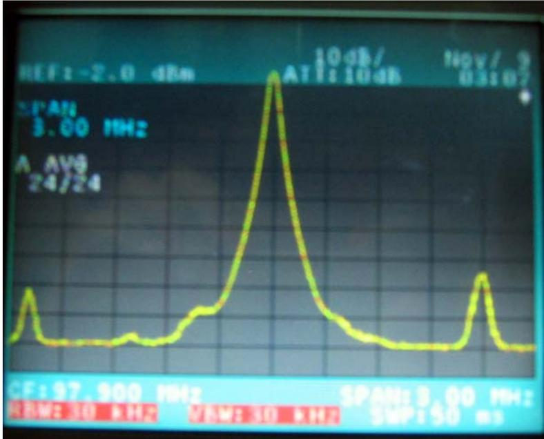
Digital image of the KBXX auxiliary transmitter, indicates response 600kHz + from center carrier. Horizontal display grid is 300kHz per division/3Mhz Span. Vertical display grid is 10db per division. 30kHz bandwidth is used during measurements. Within the limits of the linearity of the analyzer, the skirts indicate sideband energy to be more than 70db below peak carrier at 600kHz.
