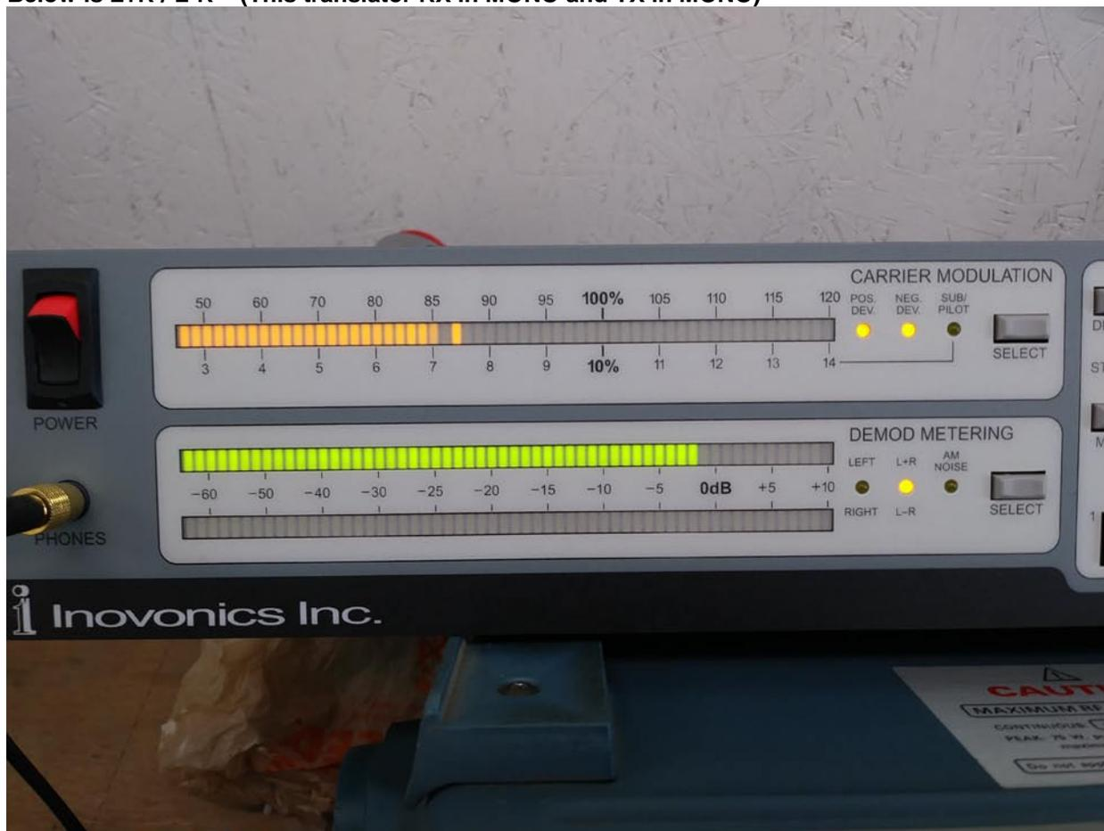
Please note that the BW Broadcast TX-50 V2 transmitter has a builtin setable limiter feature. It is currently set to a MAXIMUM of 72kHz. I tested this by adjusting the gain of the audio level on back of transmitter to EXCEED incoming level to see if this feature worked, it did and held at 72Khz DEV. I turned OFF the limiter and DEV exceeded 120% for less than 10 seconds for the test. I than turned limiter back on recalibrated the audio levels.
