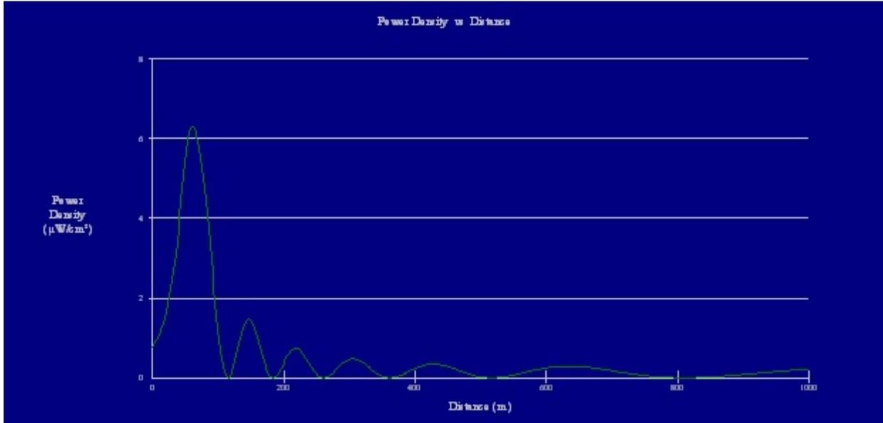
NIER Calculations at 2 meters Above Ground-Level
