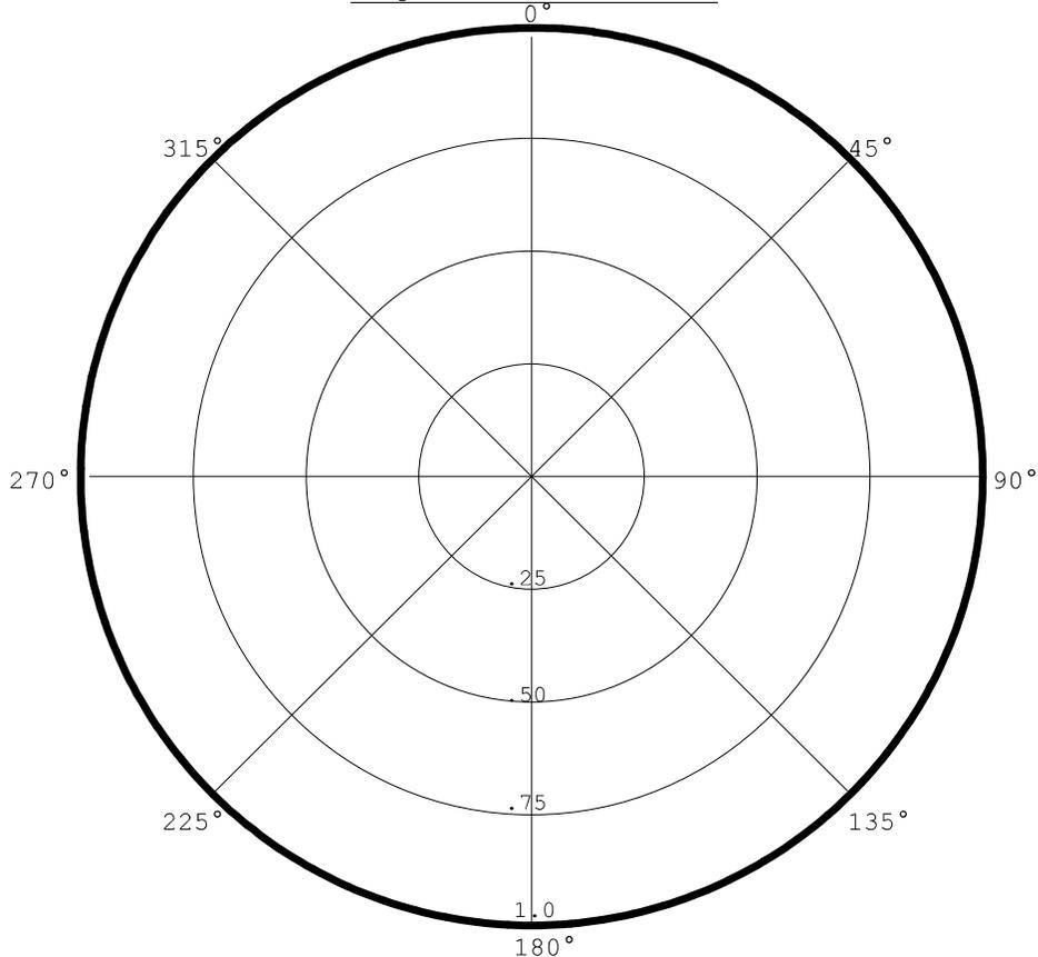
The non-directional antenna pattern will be produced by means of a Nicom Dipole BKG1/P broadcast element mounted at a 45° (degree) slant orientation to achieve horizontal and vertical polarization. The BKG1/P-1L(Slant45) Pattern is therefore a maximum composite pattern of the current horizontal and vertical broadcast patterns as notified by Nicom USA, Inc.
