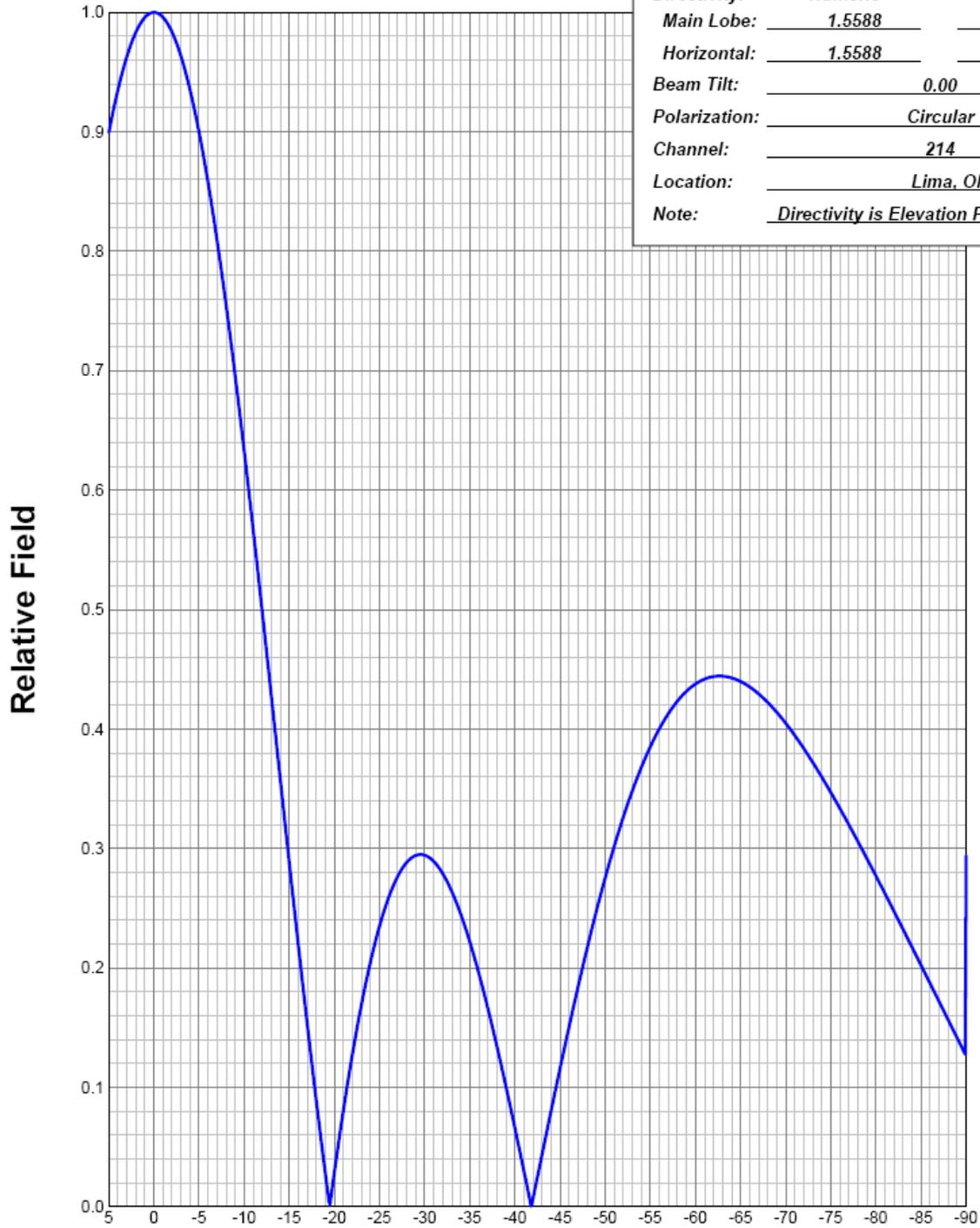
Figure 2 Calculated Vertical Plane Pattern.
