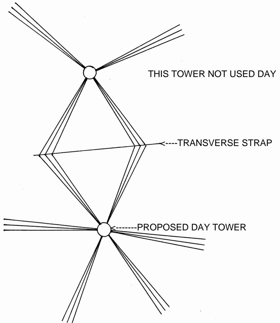
The system consists of 120 #10 soft-drawn copper wires evenly spaced 108 meters long except where truncated in a transverse strap.
