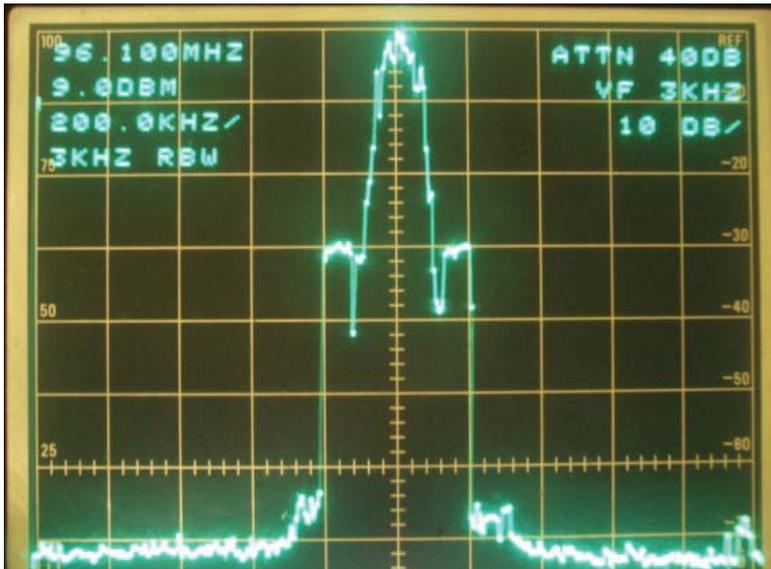
Since the resolution of the analyzer is only 70 dB, a notch filter tuned to 96.1 MHz. was placed in series with the sample element line and this photo shows there was a loss of 38 dB at 96.1 MHz.:
