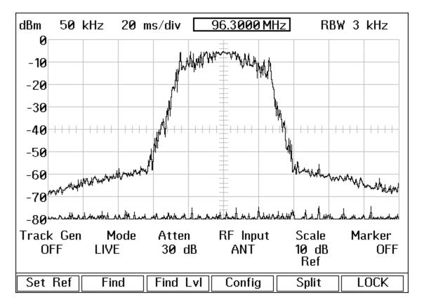
96.3 Without filtering and with 20db of external attenuation.
