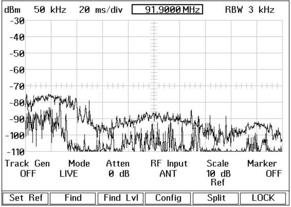
Lower Mix product with no attenuation and filters in place. Note: the signal at 91.7 is WJLF, not a mix product.
