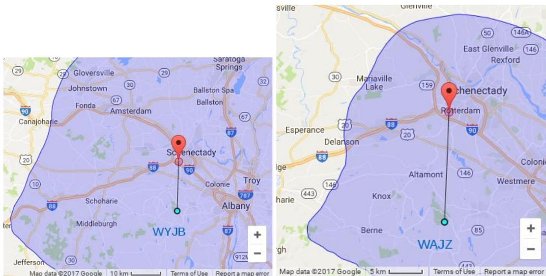
WOOS-LP seeks to escape this potential second-adjacent interference by switching to channel 255 which has no short spacings.
