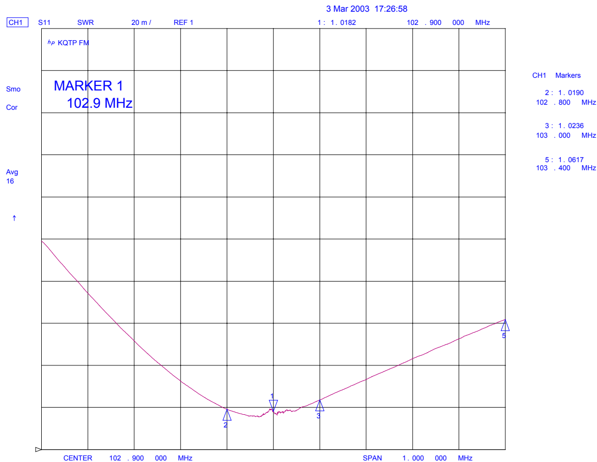
Plot # 7 Final Frequency Domain VSWR 1 Mhz Frequency Span
