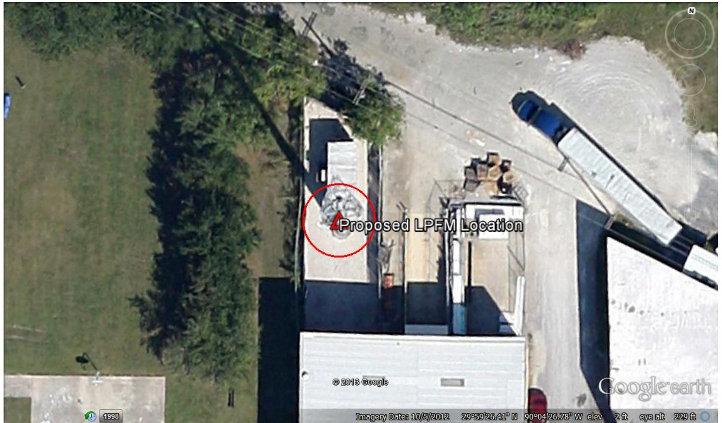
As this image demonstrates, the maximum radius would not intersect any structure except the equipment shelter at the base of the tower. However, the center of radiation is 37.2 meters AGL; therefore the interference region would be no less than approximately 33 meters, or 108 feet above ground. No portion of the interference region would impact any populated areas. A waiver of Section 73.807 of the Commission's Rules is therefore respectfully requested.
