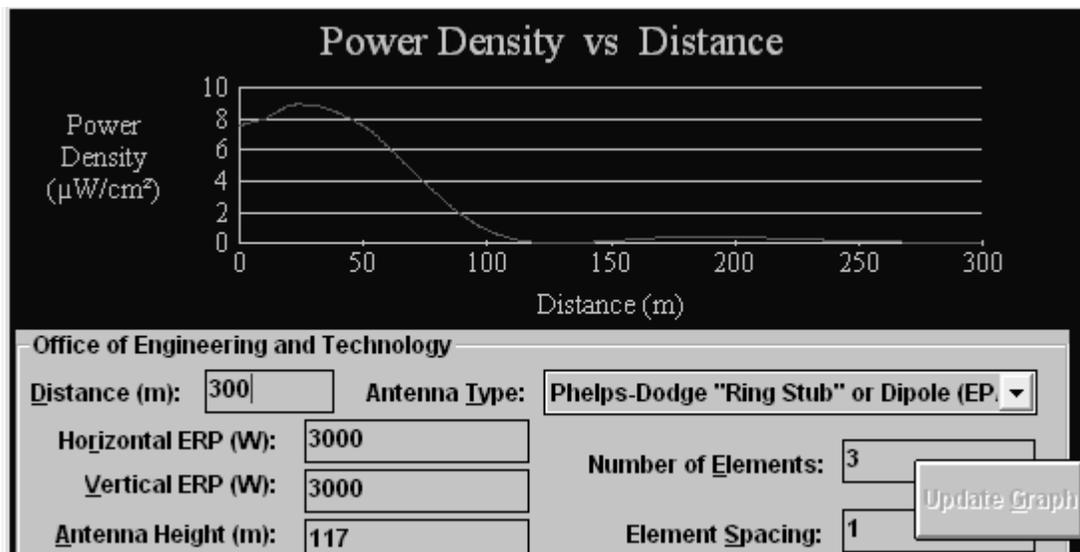
The Max Power Density was found to be 8.93429500849403  $\mu\text{W}/\text{cm}^2$  at 24 meters.
