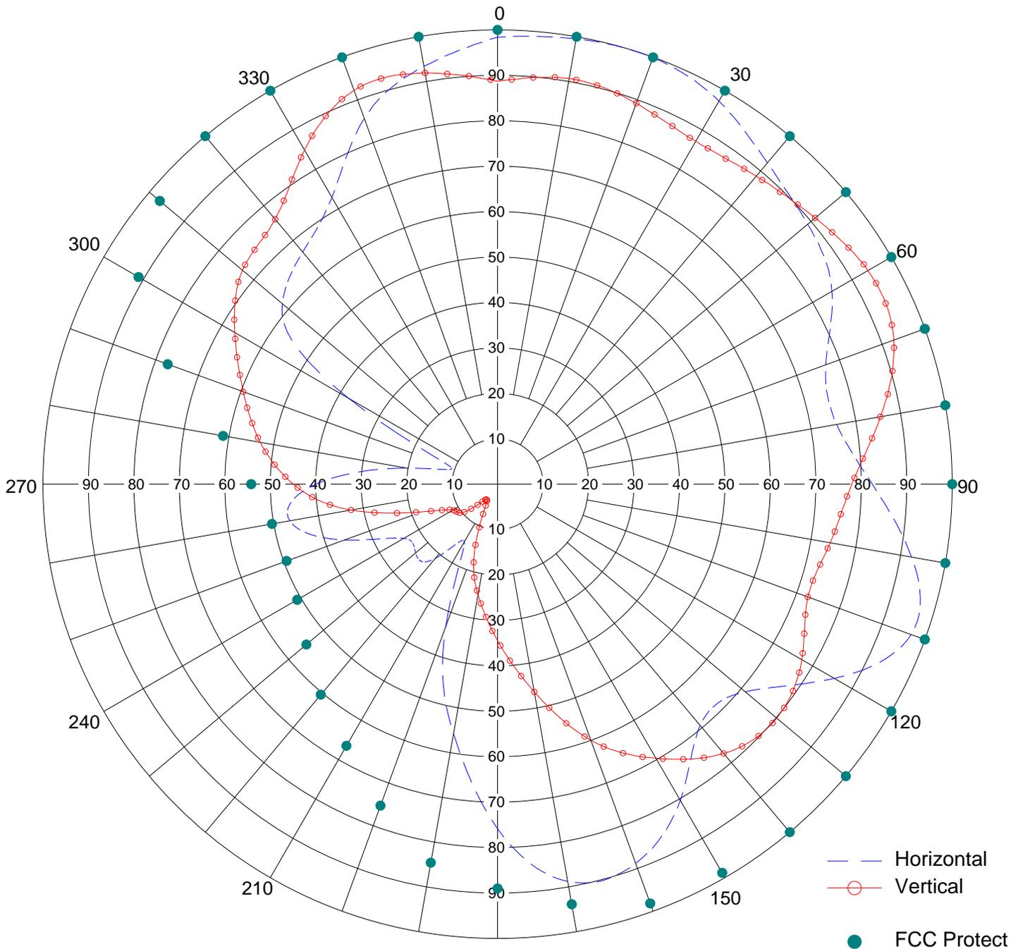
Remarks:                      Antenna Leg Mounted with one horizontal Parasitic
