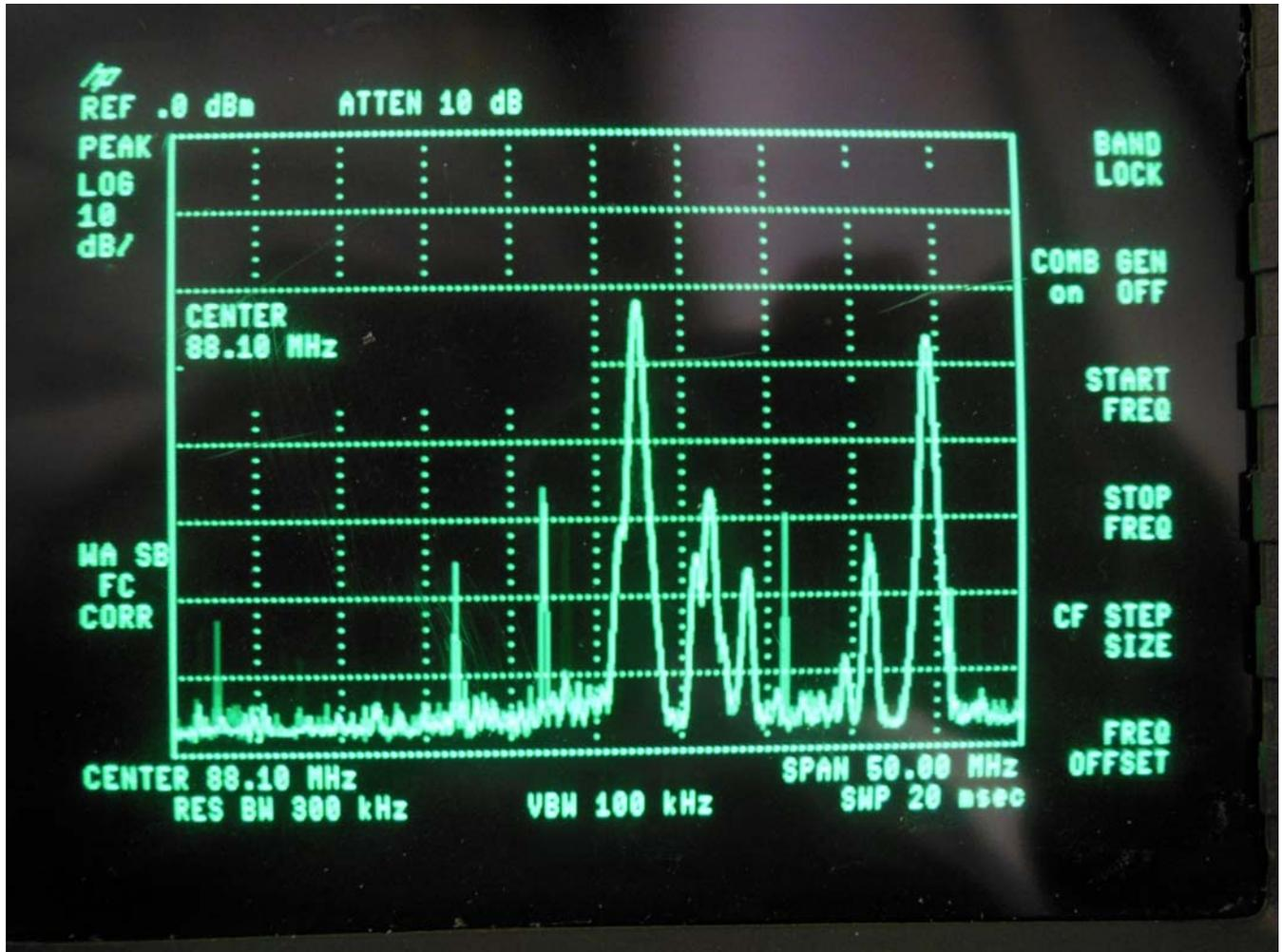
One notes several rapidly floating narrow carriers between 50 and 45 dB down, the source of which is not known. These are clearly not being caused by the KTQQ transmitter because they did not disappear when our carrier was switched off.
