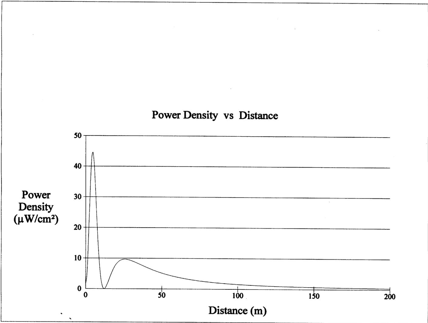
**Figure 1 - Ground Level NIER Analysis - OET FMModel**
