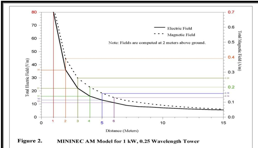
**Figure 2. MININEC AM Model for 1 kW, 0.25 Wavelength Tower**
