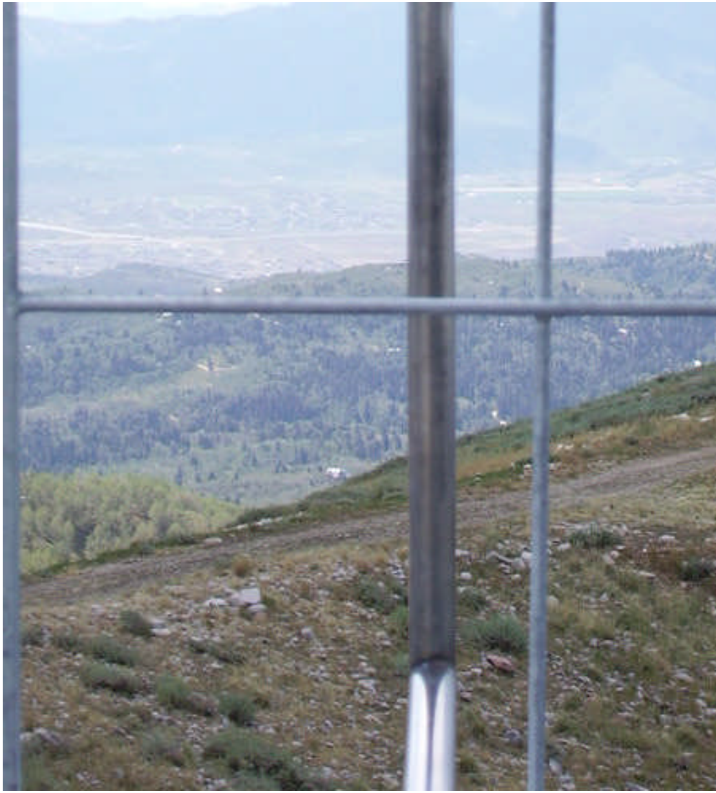
Figure 4: Radiating element of community antenna.
