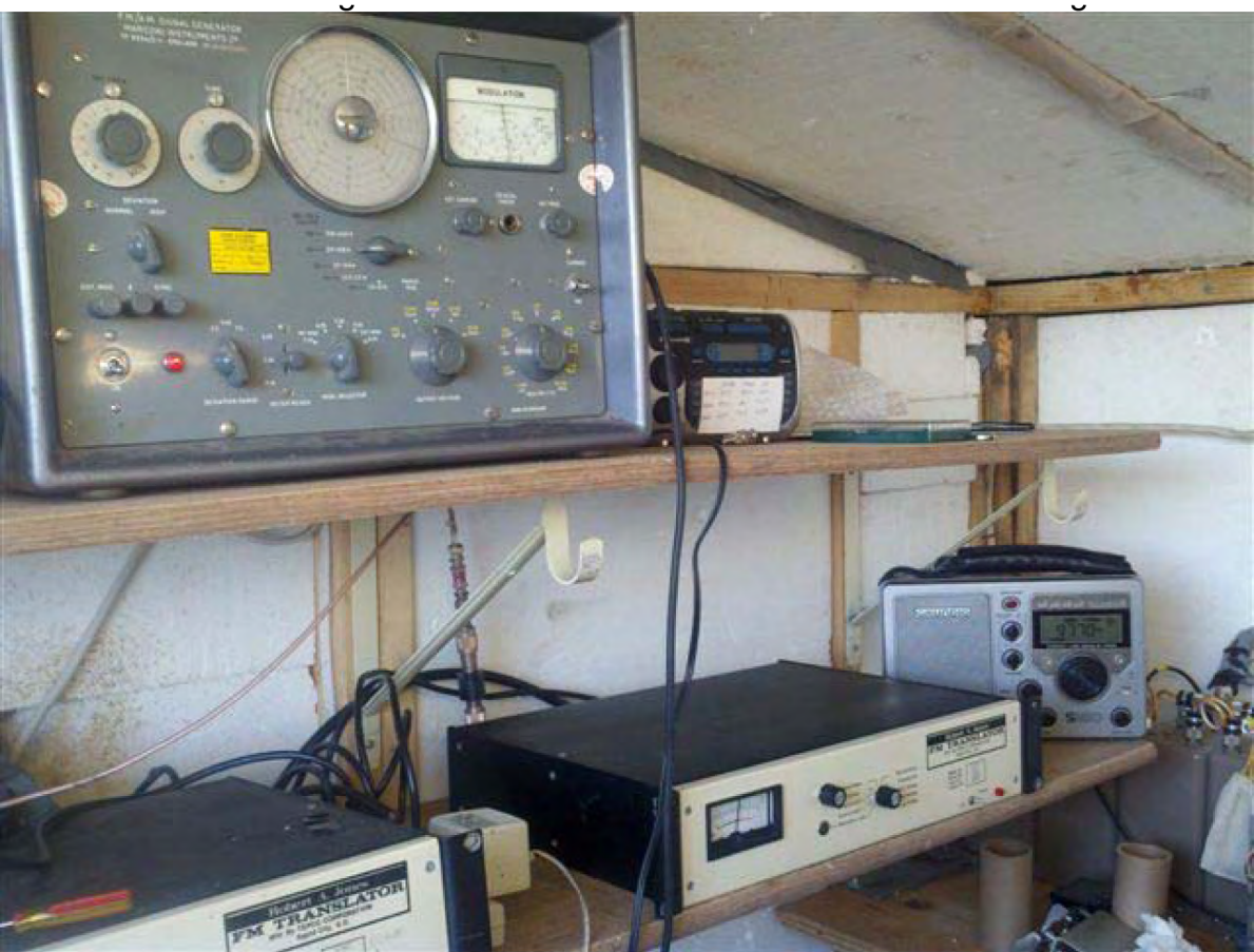
Attachment 13 View of the Signal Generator to determine received Field Strength
