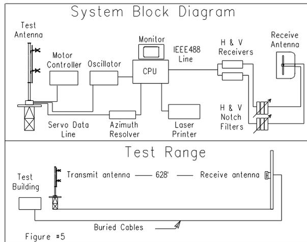
The antenna under test was operated in the transmitting mode and fed from a HP8657D signal generator. The frequency of the signal source was set at 96.7 MHz and was constantly monitored by a Rohde & Schwarz ESVD measuring receiver.
