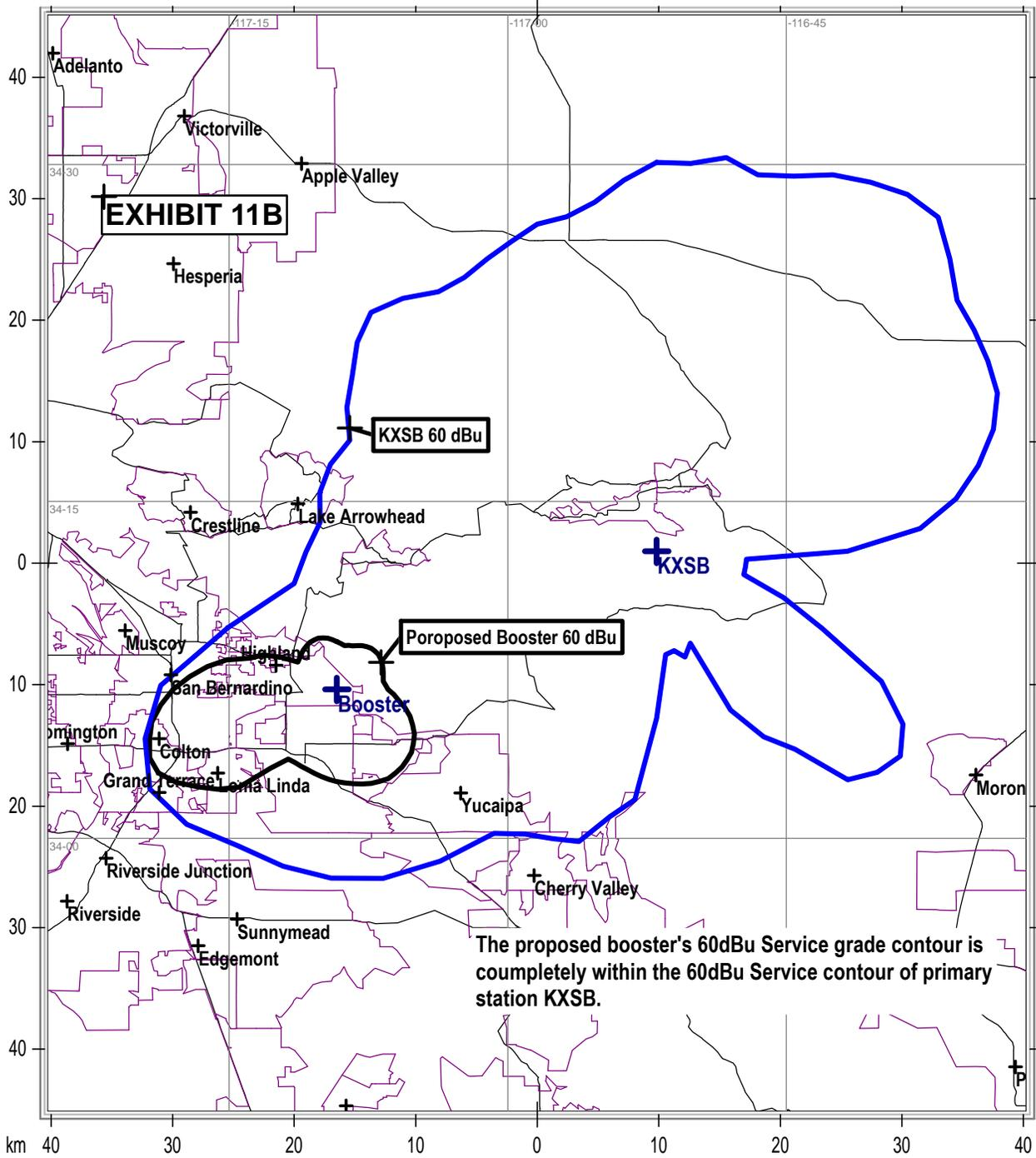
Blue = 60dBu Service Contour for KXSB, Black = 60dBu Service Contour for Proposed Booster
