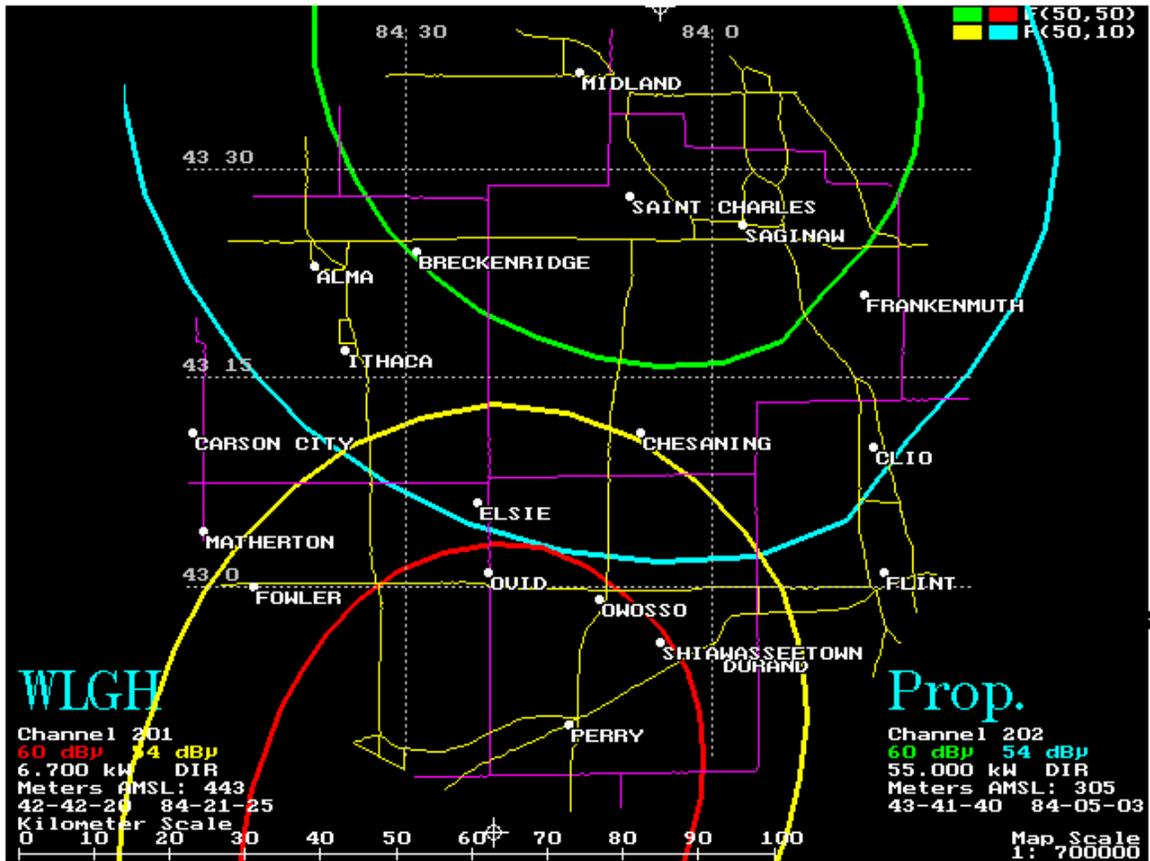
Clearance is shown with co-owned WLGH. Appropriate protected and interfering contours with respect to each station was used as required by 73.509.
