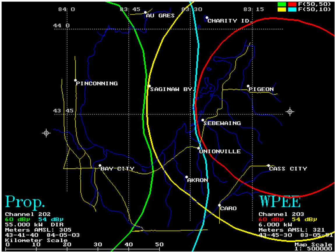
Clearance is shown with WPEE. Appropriate protected and interfering contours with respect to each station was used as required by 73.509.
