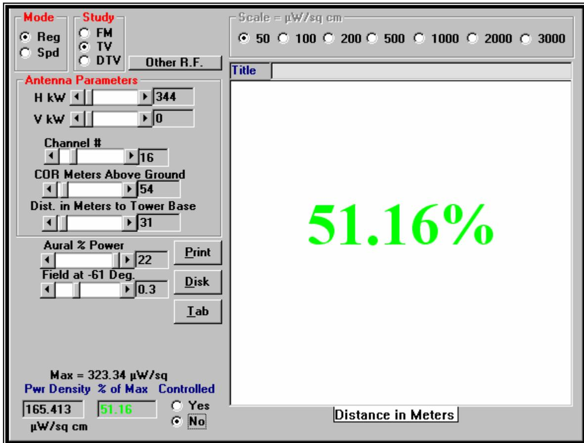
The “Dist to COR” value shown on the above graph represents the height of the antenna center of radiation above an observer on the ground who is assumed to be 2 meters in height.
