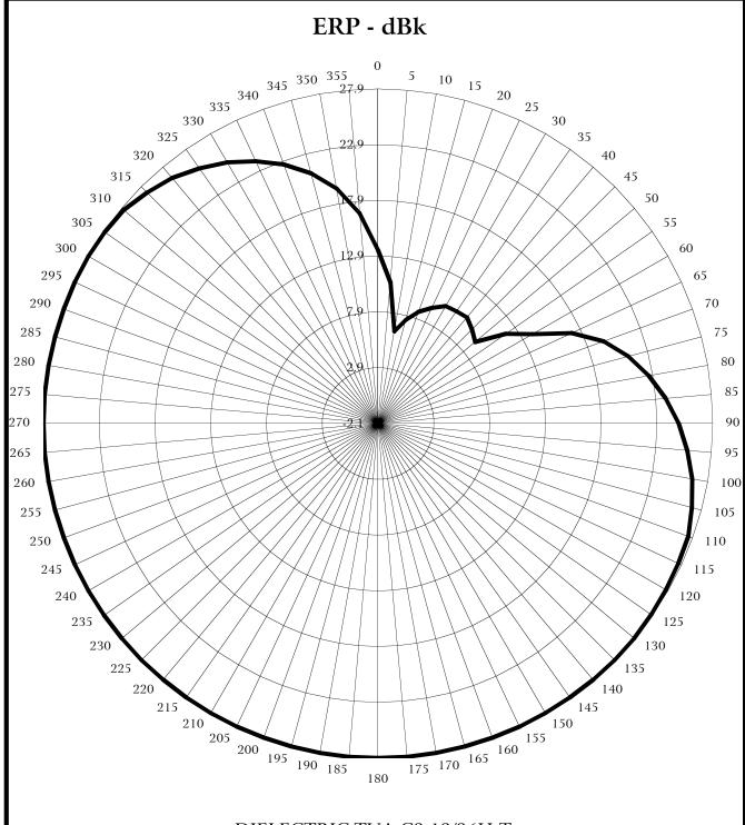
DIELECTRIC TUA-C3-12/36H-T ORIENTED WITH BEAM MAXIMA AT 130° THROUGH 300° MAXIMUM GAIN: 1.90 (2.79 DB)
