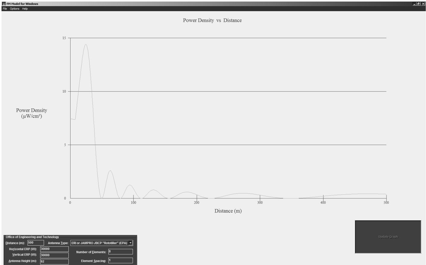
KHPO will continue to use its ERP LPX-8C, 8 Bay FM Antenna with a bay to bay spacing of 1.0 Lambda. From a height of 92 meters AGL and a ERP of 30 kW the maximum exposure at 2 meters above ground level is 14.4 uW/cm.sq at a distance of 24 meters from the base of the tower.
