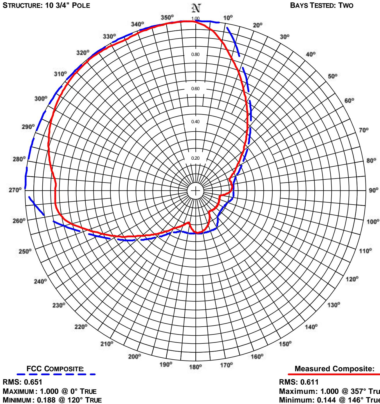
COMMENTS: Composite pattern: This pattern shows the maximum of either the H or V azimuth values. This pattern is greater than 85% of the FCC filed composite pattern BMPED-20061101ACM
