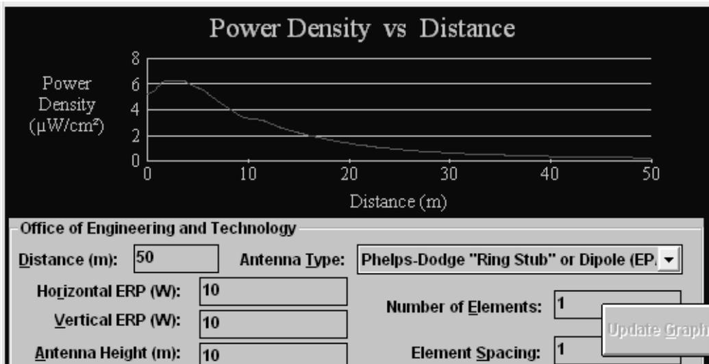
The Max Power Density was found to be 6.28264385991466  $\mu\text{W}/\text{cm}^2$  at 2.2 meters.
