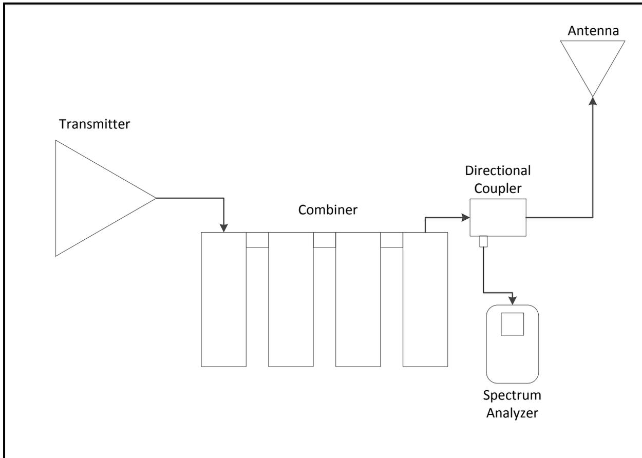
Intermodulation frequency measurement configuration
