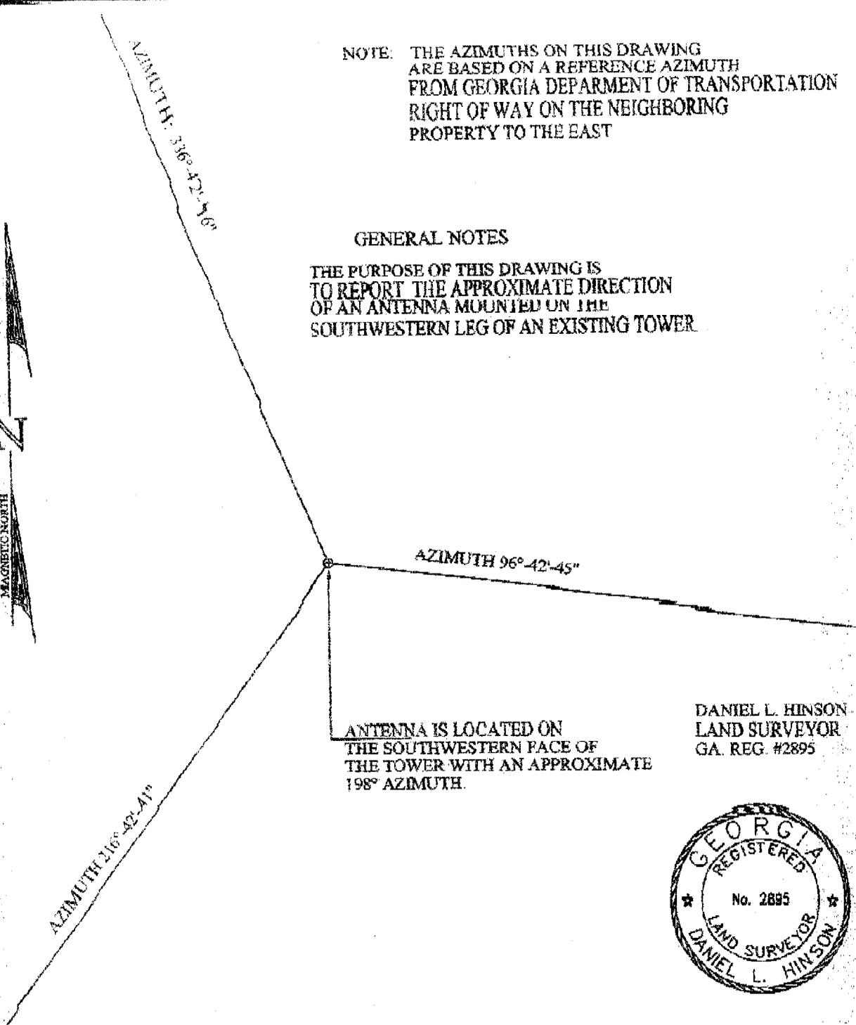
ANTENNA IS LOCATED ON THE SOUTHWESTERN FACE OF THE TOWER WITH AN APPROXIMATE 198° AZIMUTH.
