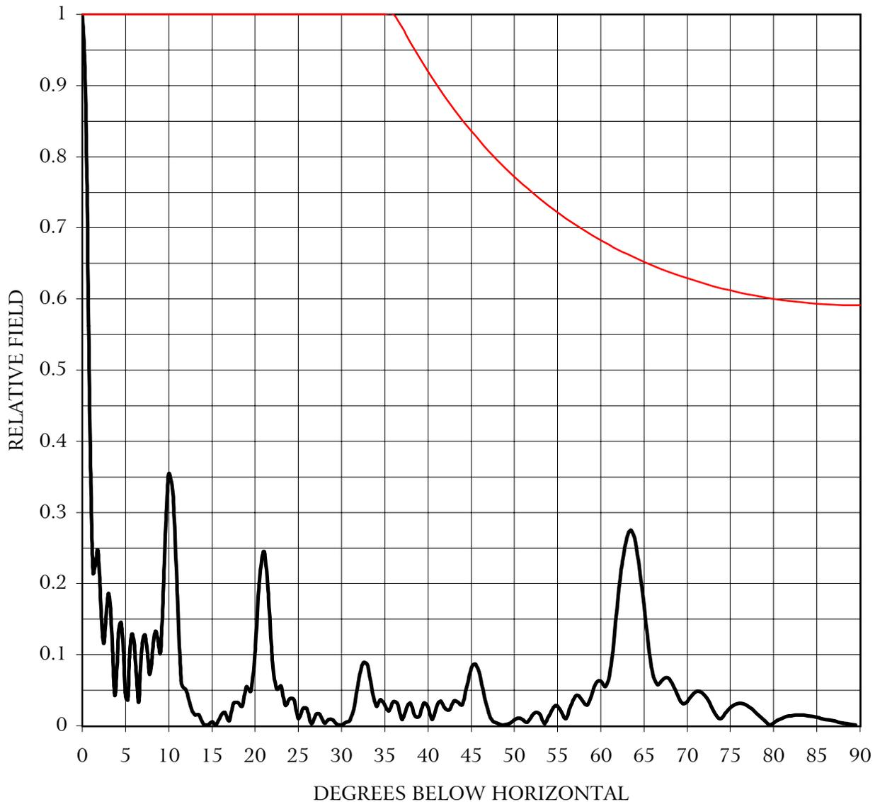
— Represents the relative field of the proposed antenna with respect to the degrees below the horizontal plane.
