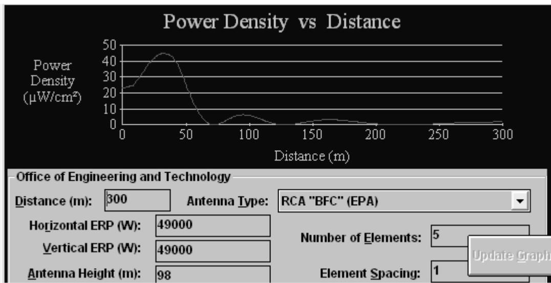
The Max Power Density was found to be 44.848959123701  $\mu\text{W}/\text{cm}^2$  at 32.4 meters.
