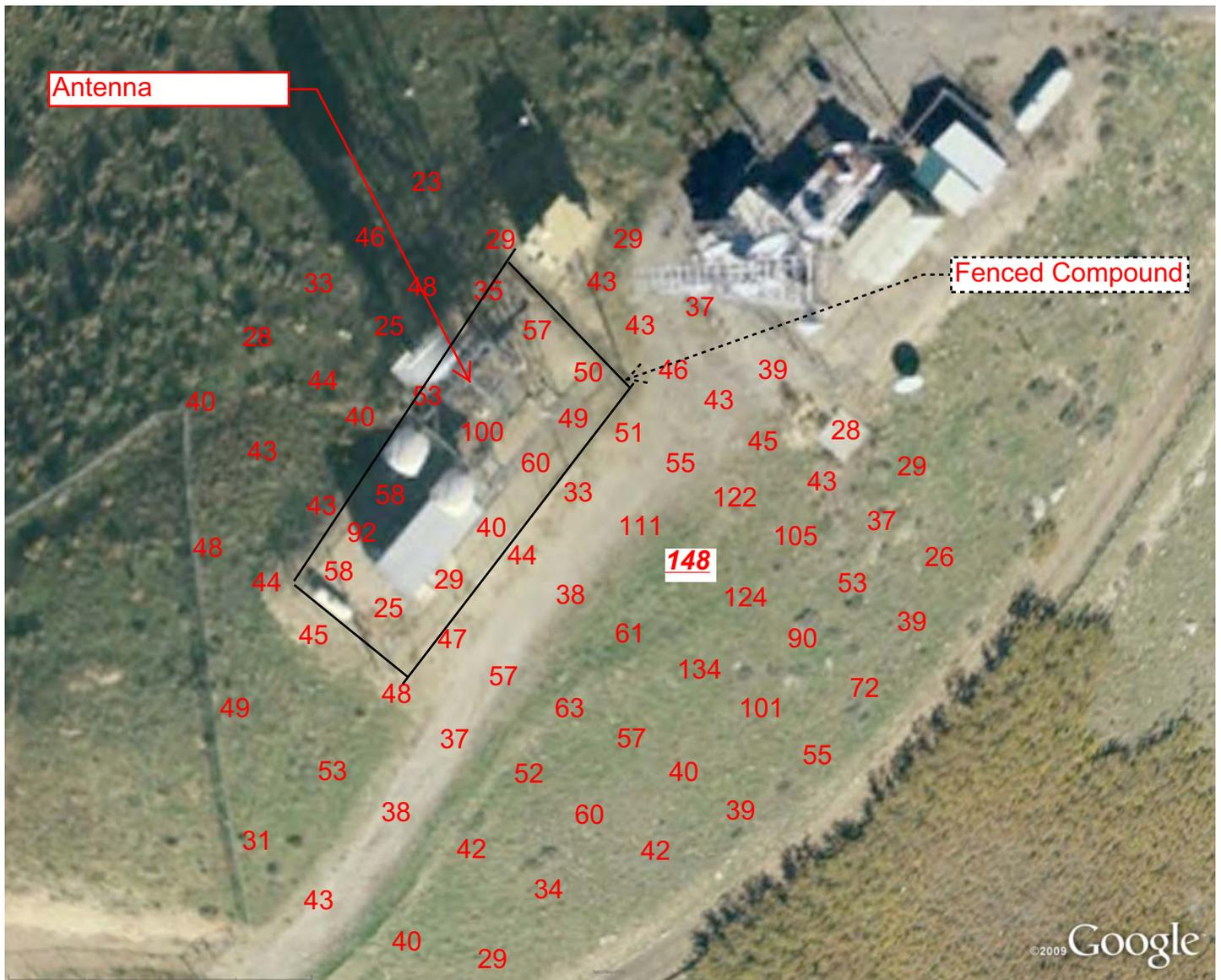
All Values in Microwatts per Square Centimeter where 200 would exceed the Uncontrolled Standard for ANSI downward RFR. The highest recorded value, as highlighted on the map, was 148  $\mu\text{W}/\text{cm}^2$ , or 74% of the Uncontrolled Standard measured at a location 55 feet in front of the antenna in its peak azimuth lobe. Therefore, the site complies with the Uncontrolled Standard at all locations.
