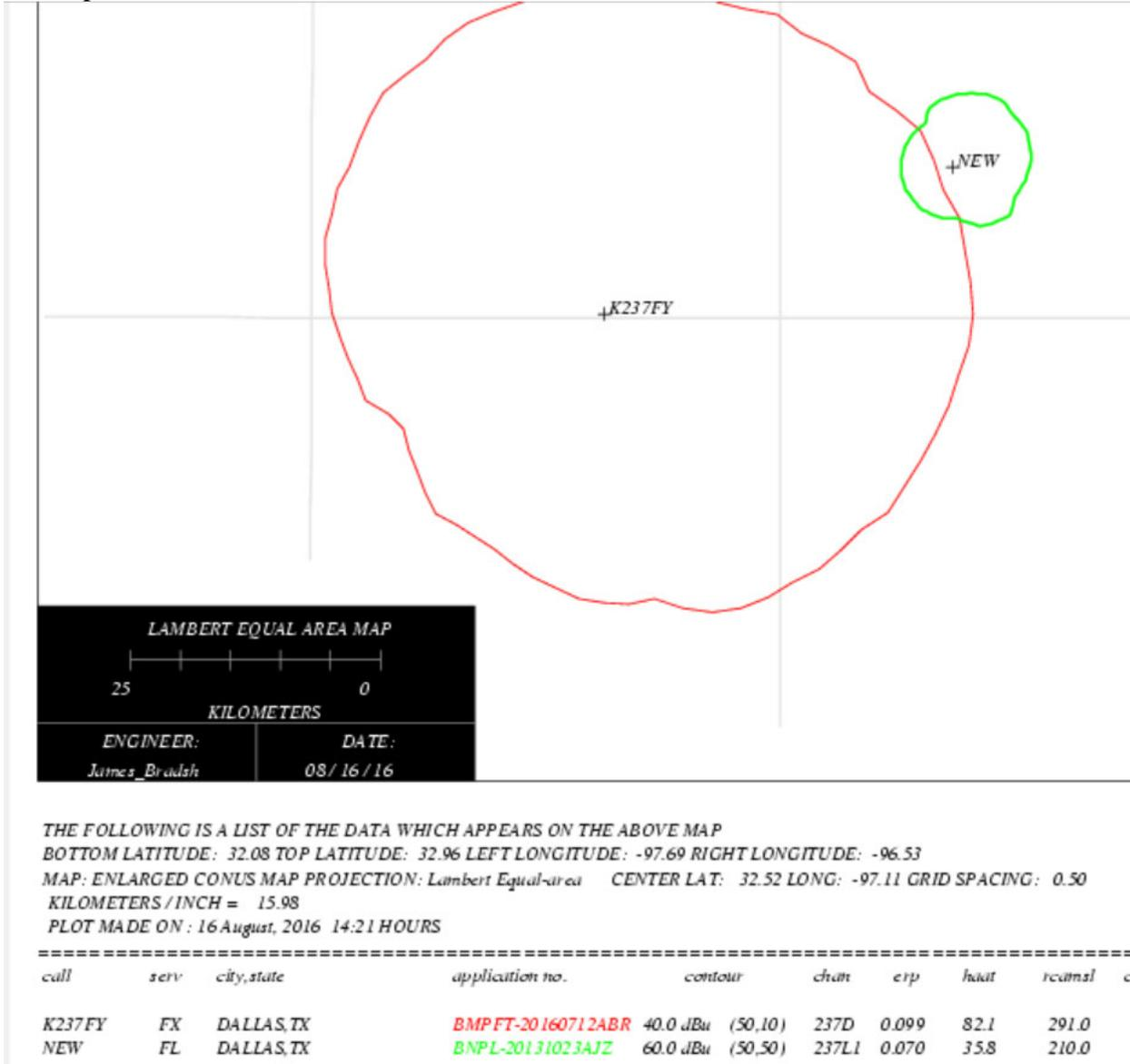
Red contour: K237FY, BMPFT-20160712ABR – 40 dBu interfering contour
