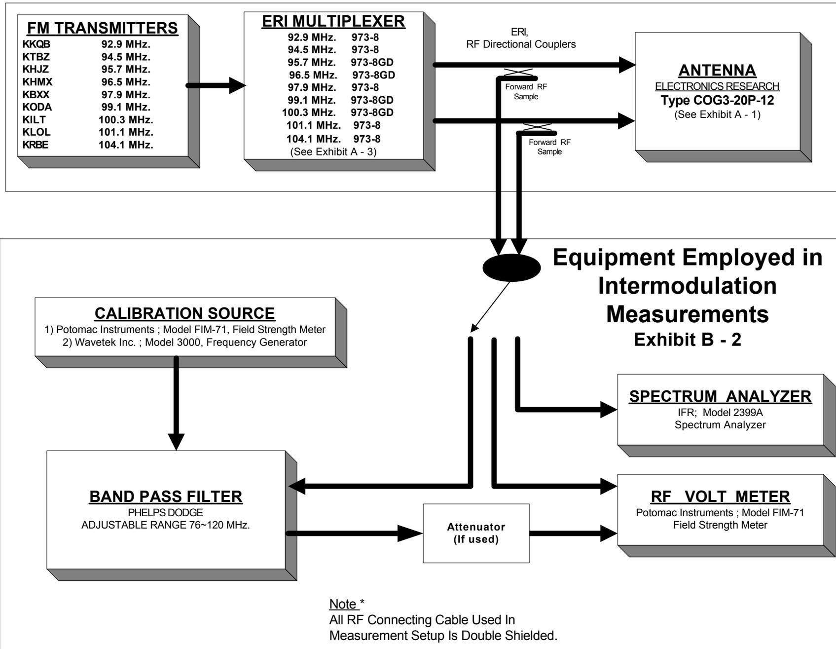
Broadcasting Scheme and Equipment Employed in Intermodulation Measurements
