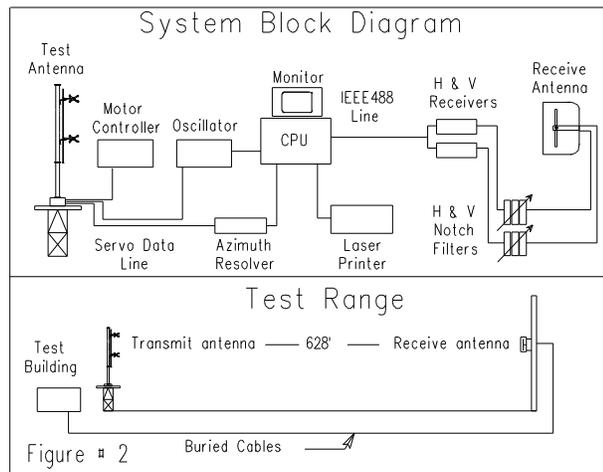
approximately 30 feet above ground. The turntable is equipped with a motor drive and a US Digital angle position indicator. The resolution of this angle position indicator is one-hundredth of a degree.
