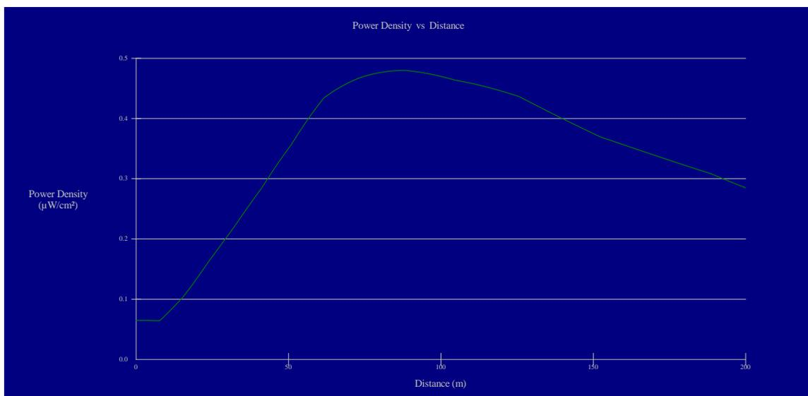
The FCC's FM Model program does not have a model for the Scala Log Periodic antenna. The proposed antenna for K277CE will be a vertically polarized Scala Log Periodic. The actual level shown is 0.48 microwatts/centimeter squared, well below the 200 microwatts allowed. A LP antenna would exhibit even less radiation exposure on the ground.
