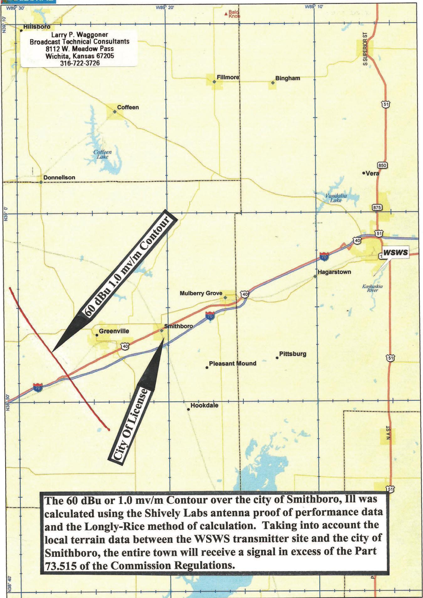
**The 60 dBu or 1.0 mv/m Contour over the city of Smithboro, Ill was calculated using the Shively Labs antenna proof of performance data and the Longly-Rice method of calculation. Taking into account the local terrain data between the WSWS transmitter site and the city of Smithboro, the entire town will receive a signal in excess of the Part 73.515 of the Commission Regulations.**
