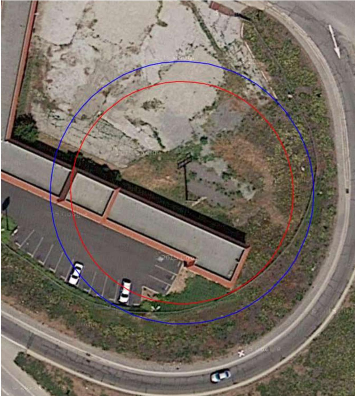
The **BLUE CURVE** is the 30 meter radius of the interference contour at the center of radiation. The **RED CURVE** is the 25.7 meter radius of the interference contour as it reaches ground level. The structure is a two-story occupied hotel. Due to the horizontal pattern of the proposed antenna, interference to KRAY-FM will be above the occupied structure and will not penetrate the structure itself.
