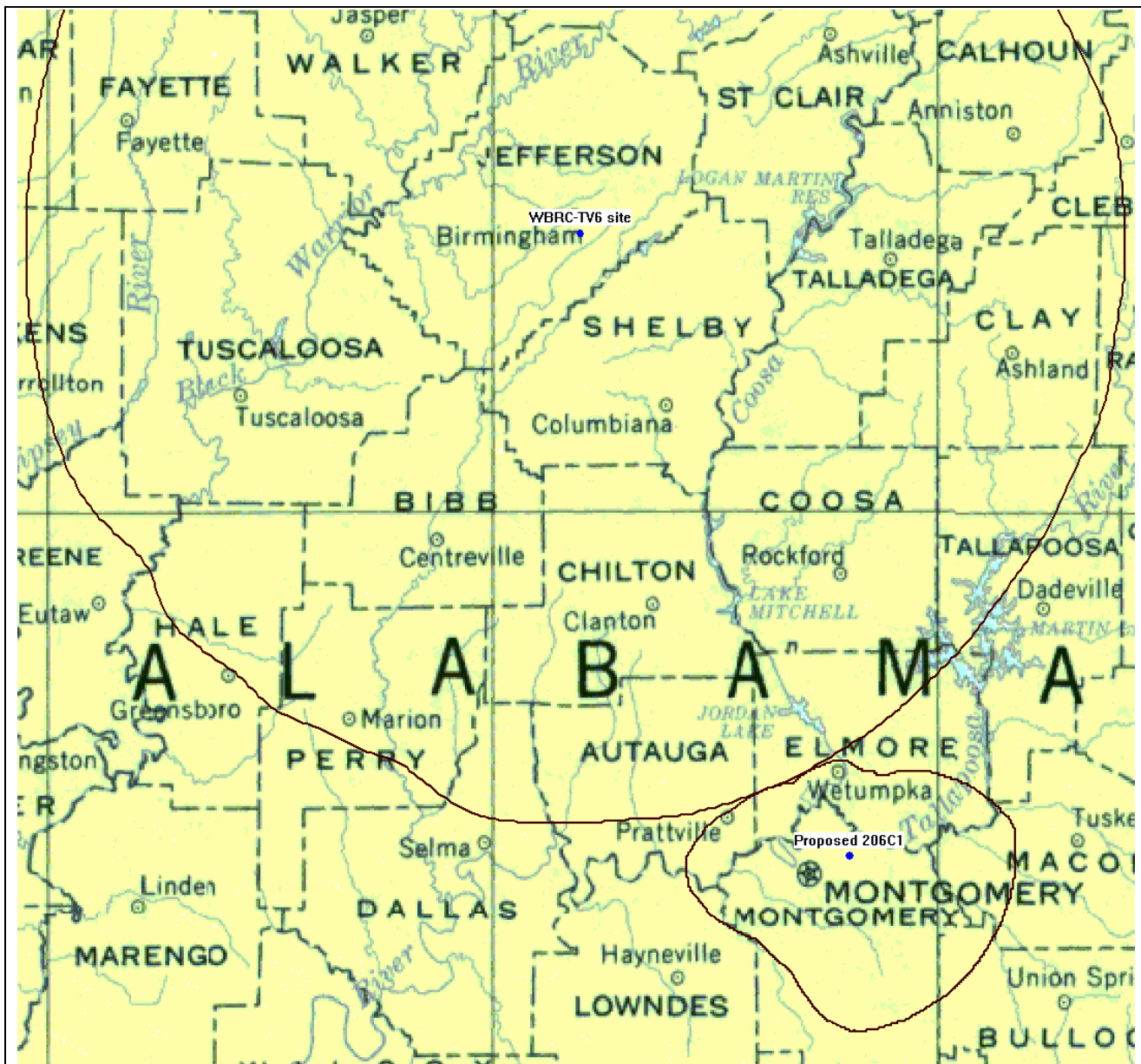
Figure 3: Proposed 206C1 40:1 63.5dBu Interfering Contour vs TV Channel 6 Grade B Protected Contour
