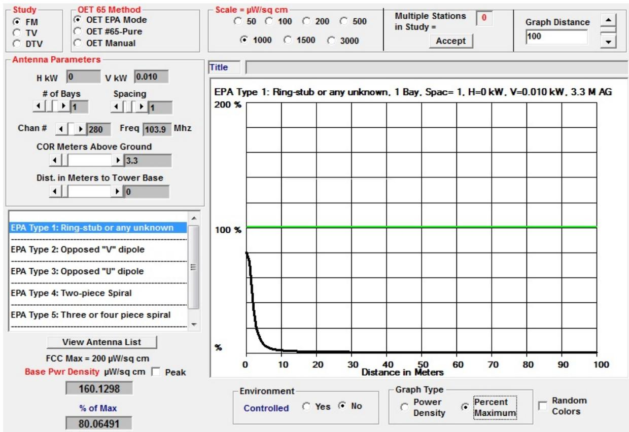
RF-Haz also shows that for controlled access 2 meters AGL (above the height of the public) will not exceed 17% of the OET radiation limit for a controlled environment, such as is the case for the secure, fenced-in tower compound.
