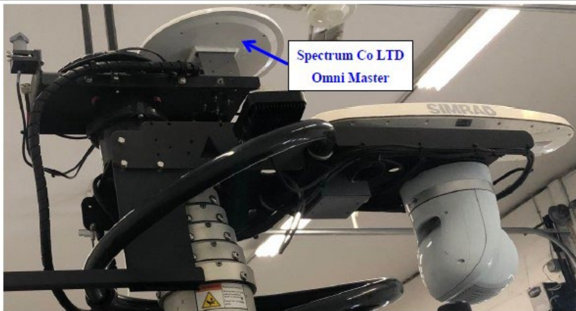
Figure A2-3b UHF omni-directional antenna mounted on top of field test van's mast.
