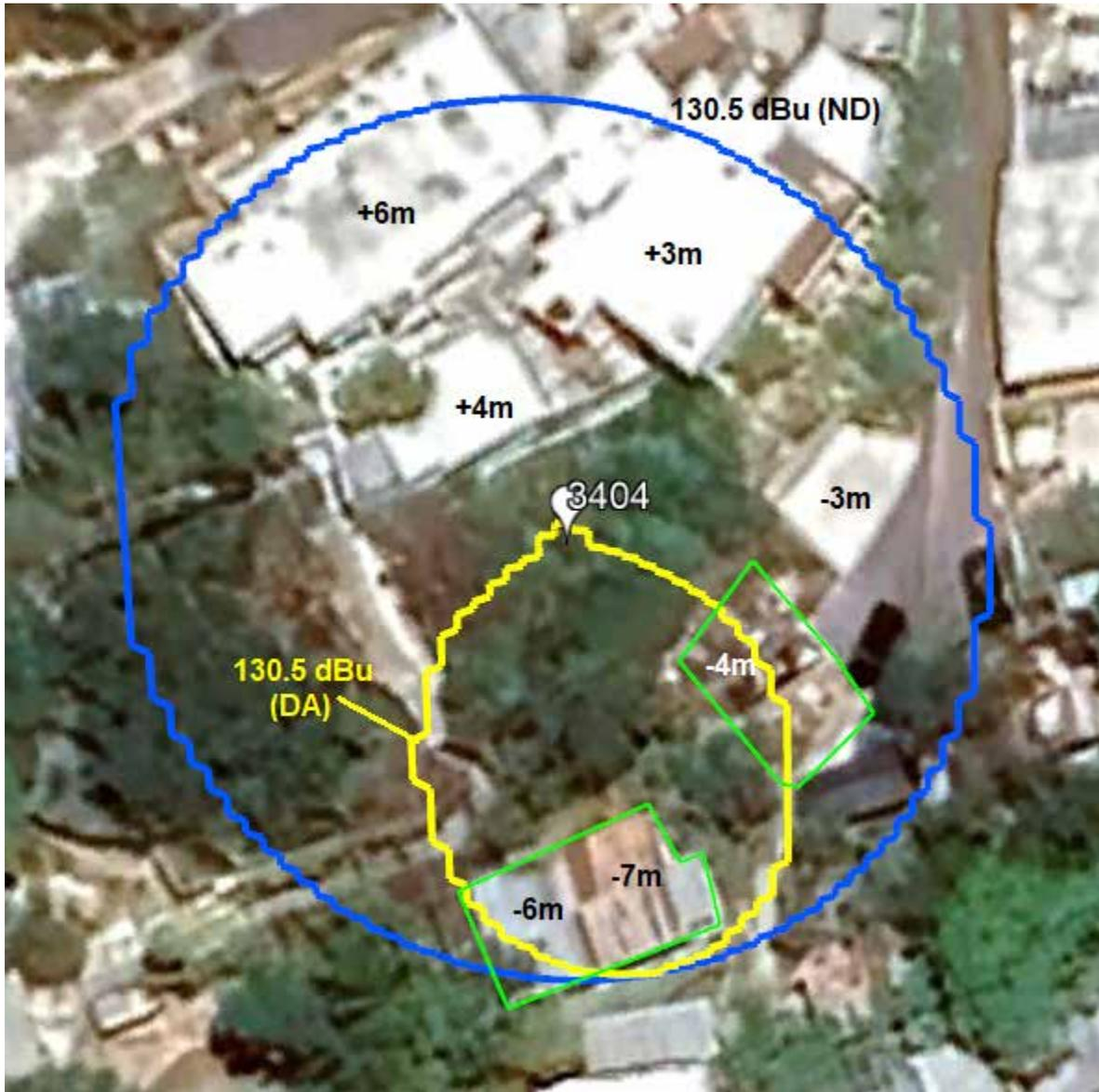
Blue curve = 130.5 dBu interfering contour if nondirectional.
