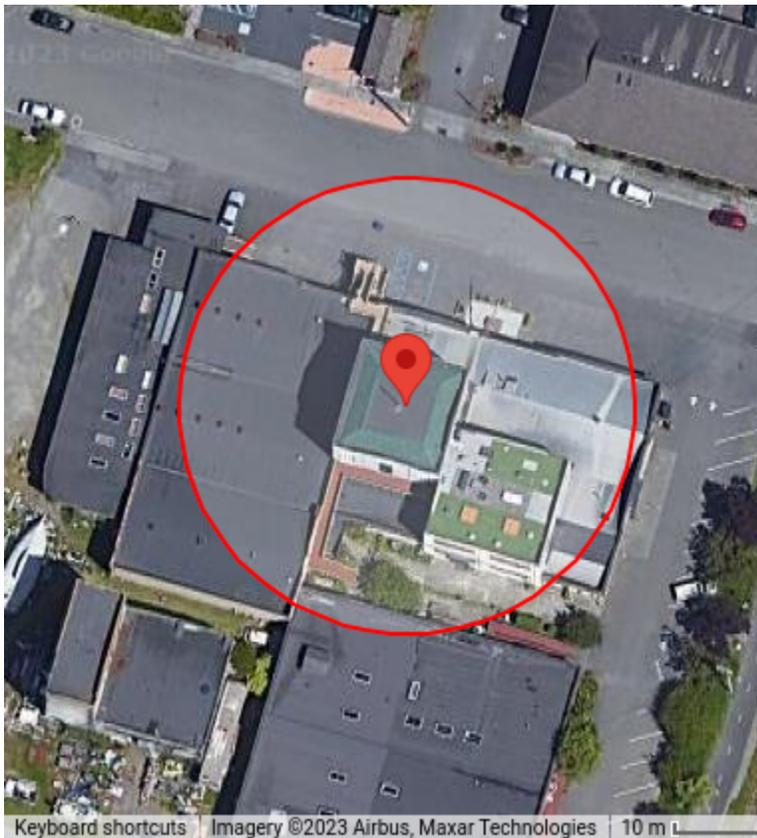
The proposed Norwalk NWE-34 antenna is to be mounted at 26 meters AGL, 9 meters above a tower rooftop. Within the building complex, the top floor elevation is 13 meters AGL. By virtue of its elevation pattern, the NWE-34 reduces the downward interference contour distance from 26.1 to 10.5 meters below the antenna resulting in a potential interference floor of  $26 - 10.5 = 15.5$  meters AGL which is 0.5m above the heads of people on the top floor.
