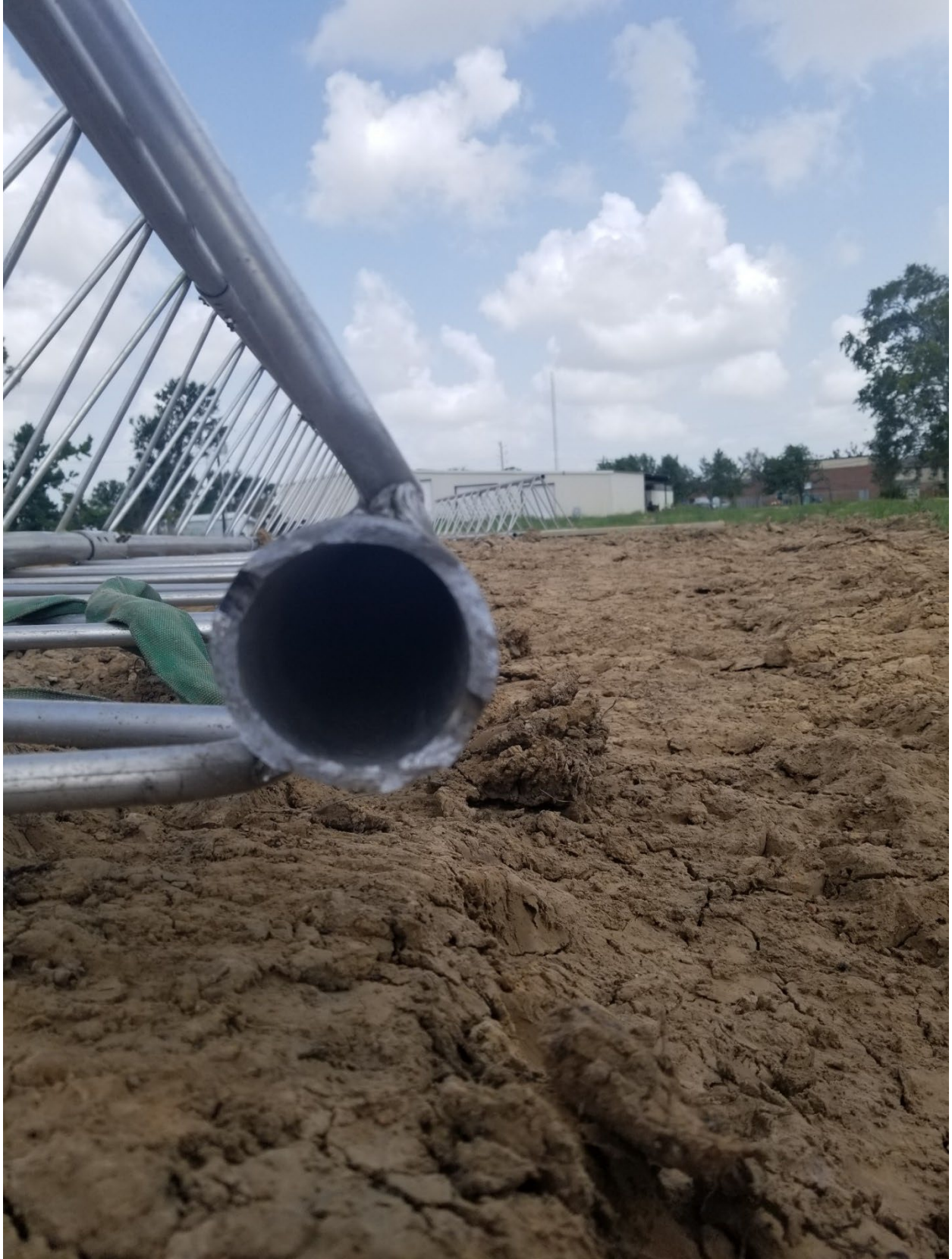
Broken tower leg that caused the second silent period.
