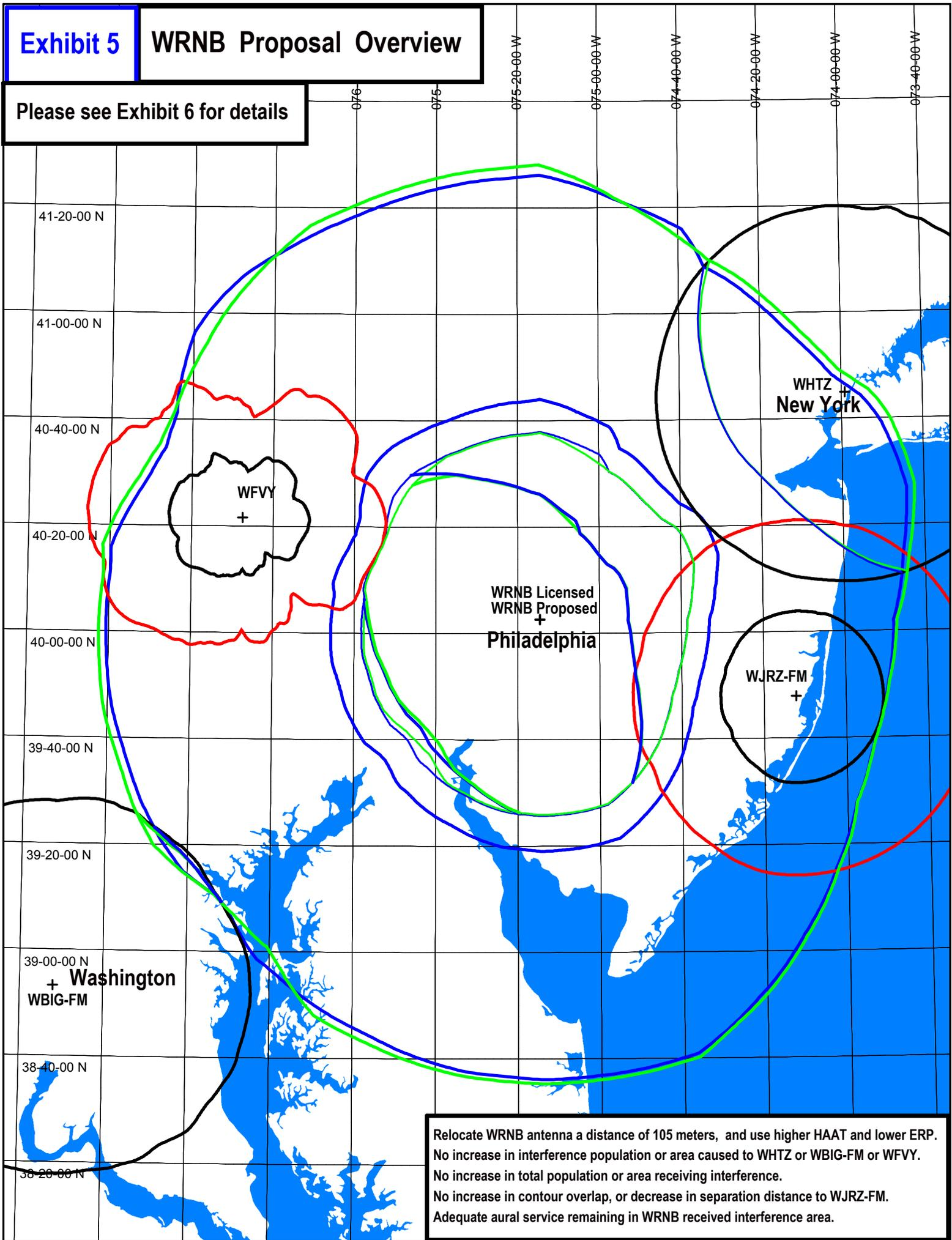
Relocate WRNB antenna a distance of 105 meters, and use higher HAAT and lower ERP.
