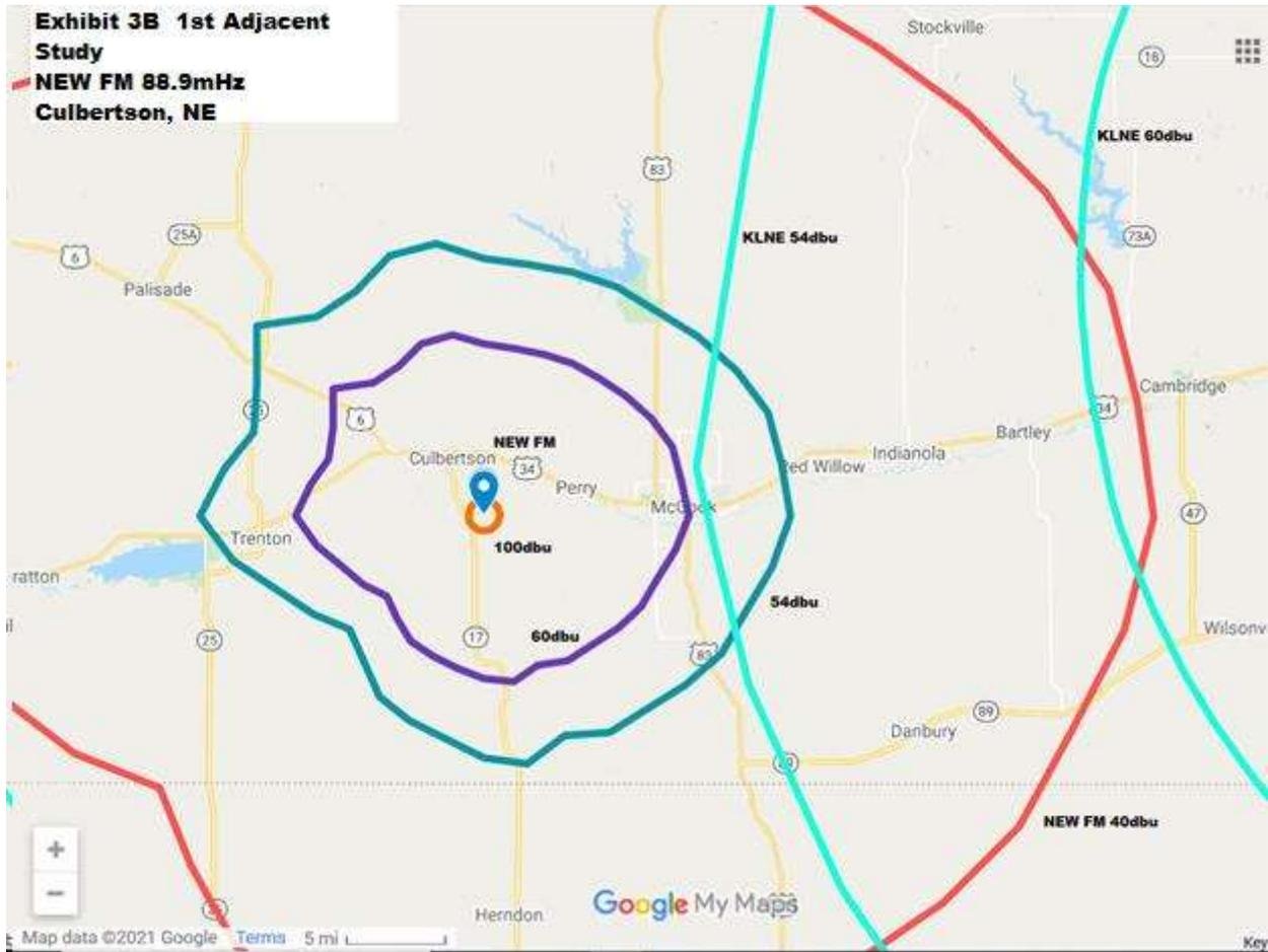
On this map we see that 1<sup>st</sup> Adjacent KLNE, Lexington's 54dbu contour is not crossed by the NEW FM 60dbu contour and likewise the KLNE 60dbu is not crossed by the 54dbu contour of the new FM. (The red 40dbu contour is irrelevant to this map)
