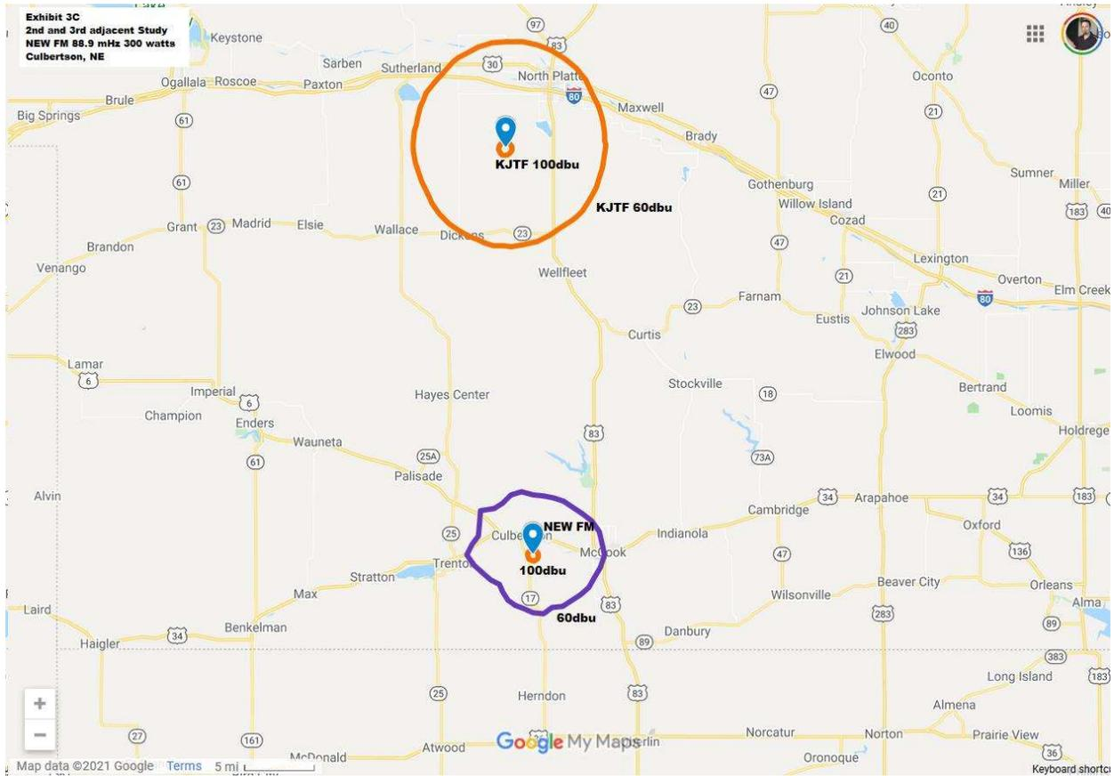
The closest 2<sup>nd</sup> adjacent FM station is KJTF, North Platte. Not even close to overlapping 100dbu and 60dbu in either direction. No 3<sup>rd</sup> adjacent stations are within range of the study.
