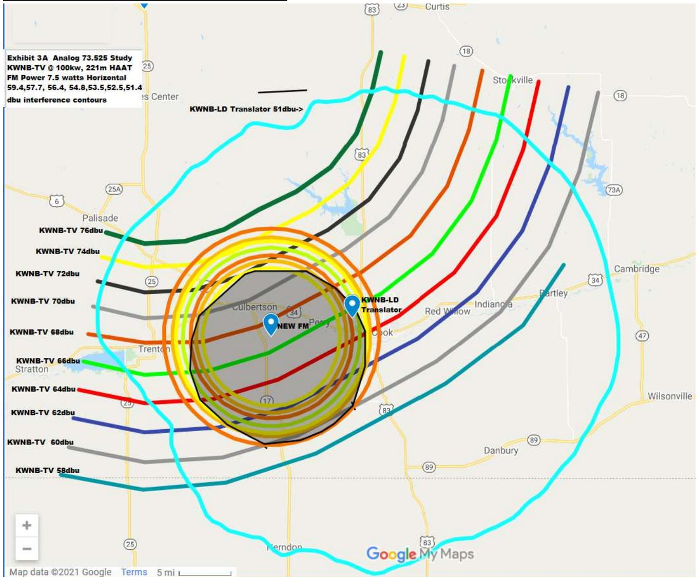
As shown in this exhibit there are overlapping interference contours. The applicant counts 2,206 persons within the Interference Nexus using the 100kw analog method of calculation for KWNB-TV. This is under the 3000 allowed. The population counts were done in accordance with FCC procedure, taking US Census subdivision block maps and interpolating for county subdivisions where 100% was not covered.
