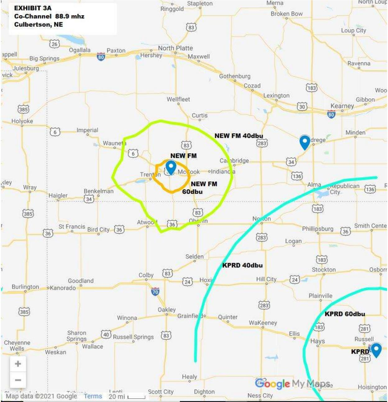
As can be seen there is nothing close to overlap on the co-channel map. The only station close is KPRD in Hays, KS, shown here. 40dbu and 60dbu contours shown.
