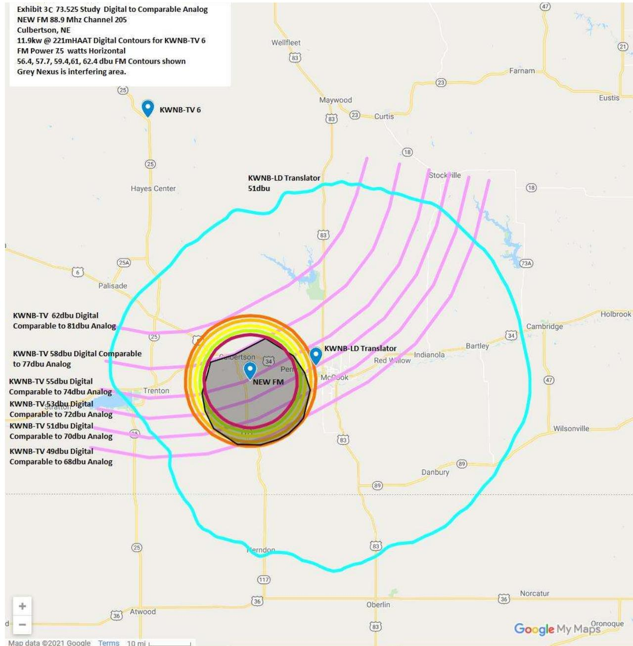
Fm Power is at 7.5 watts on all of the 73.525 study maps. KWNB-TV Power is at 11.9KW their current authorized digital power. They have a permit to increase power to 45KW. This would make the area of interference even less by pushing out the KWNB-TV Contours further.
