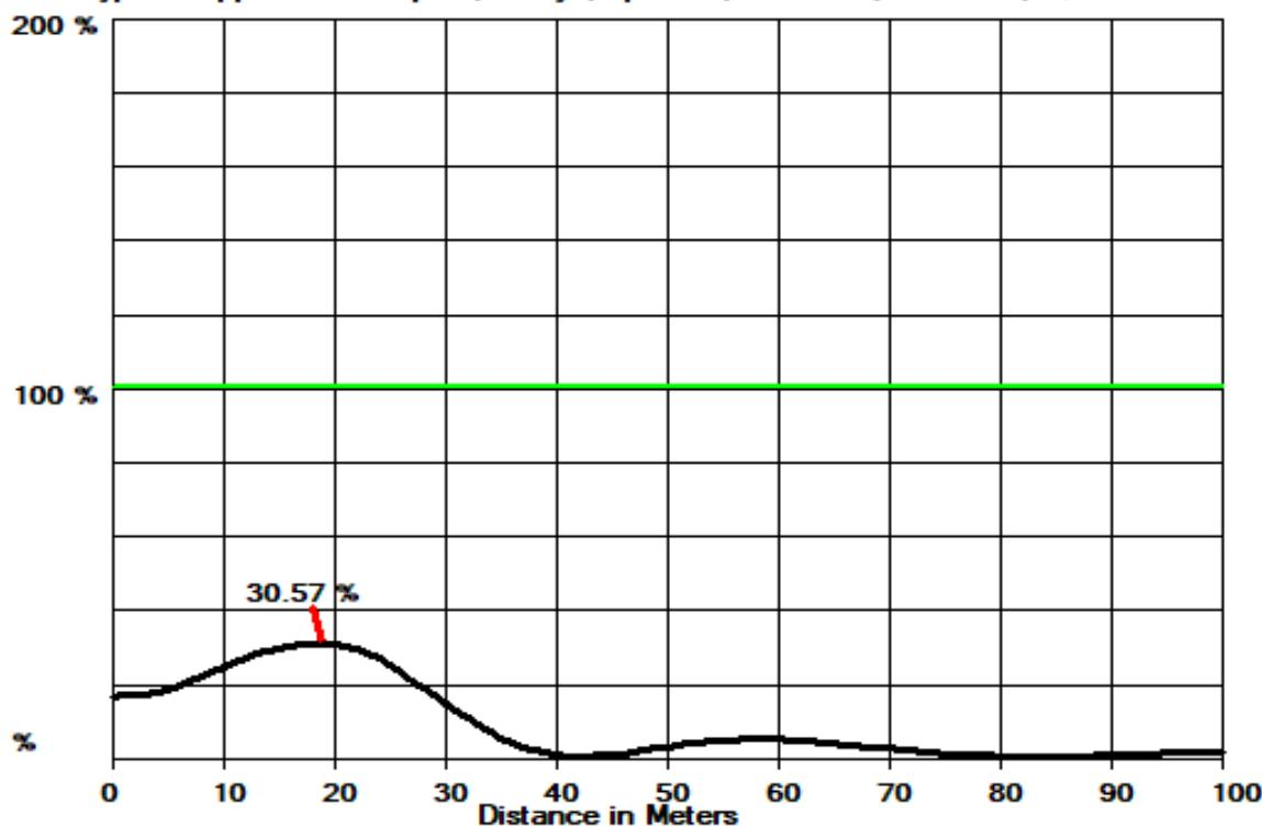
HORZ. DISTANCE FROM FM RADIATOR VS POWER DENSITY (Microwatt/Square cm)
