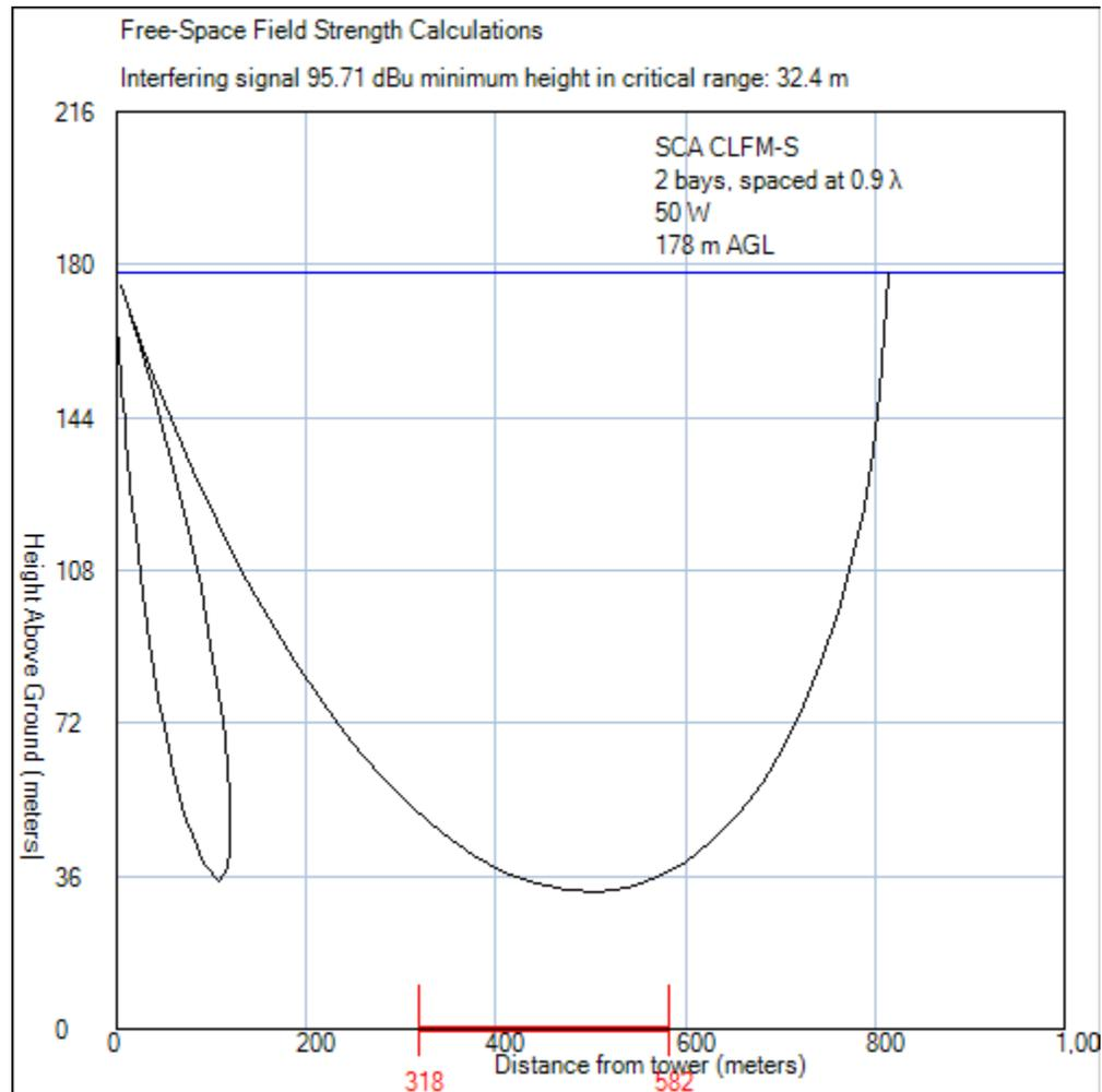
With a minimum elevation above ground of 32.4 m, the interfering signal will clearly not impact any occupied area.
