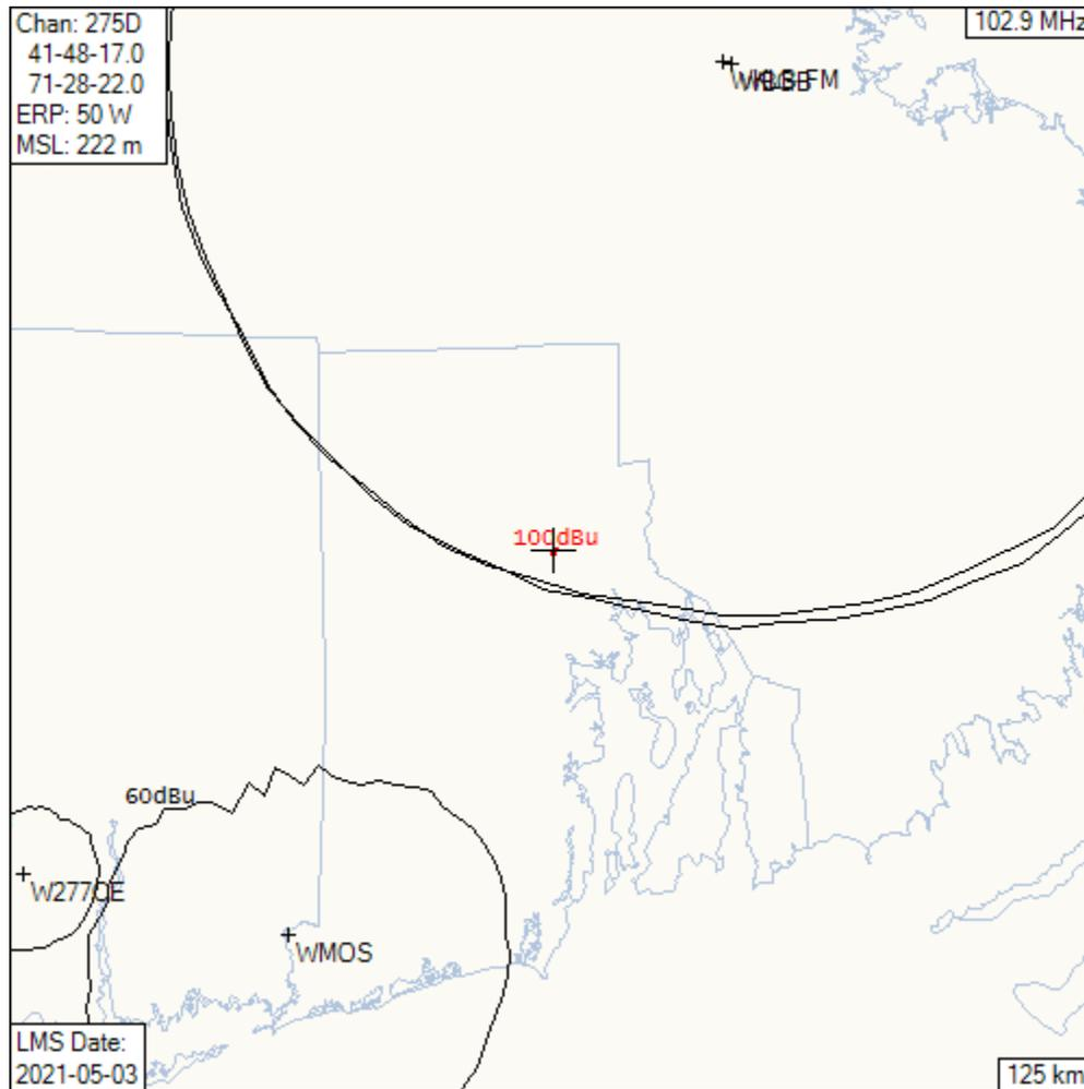
The proposed location is within the protected contours of WKLB (55.71 dBu at the proposed site) and WBGB (56.04 dBu at the proposed site).
