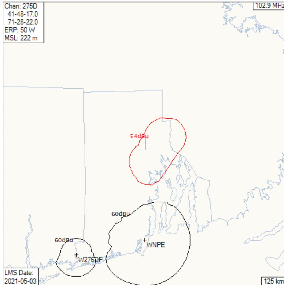
WNPE is Class A, and W276DF is a translator. Both are protected to the 60 dBu f(50,50) contour. The interfering contour is 54 dBu f(50,10).
