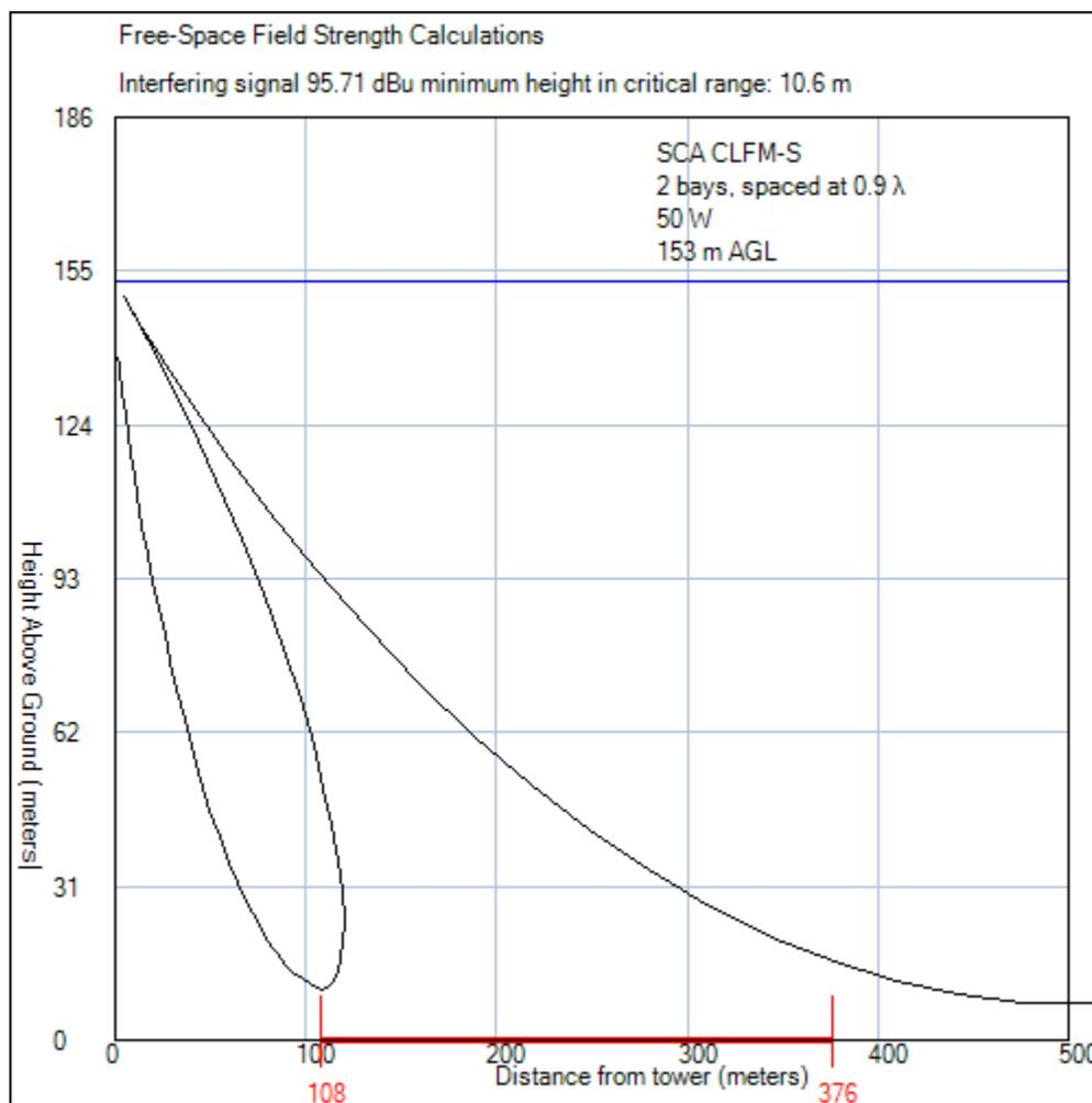
The interfering signal level of 95.71 dBu is at least 10.6 m above ground anywhere in this area.
