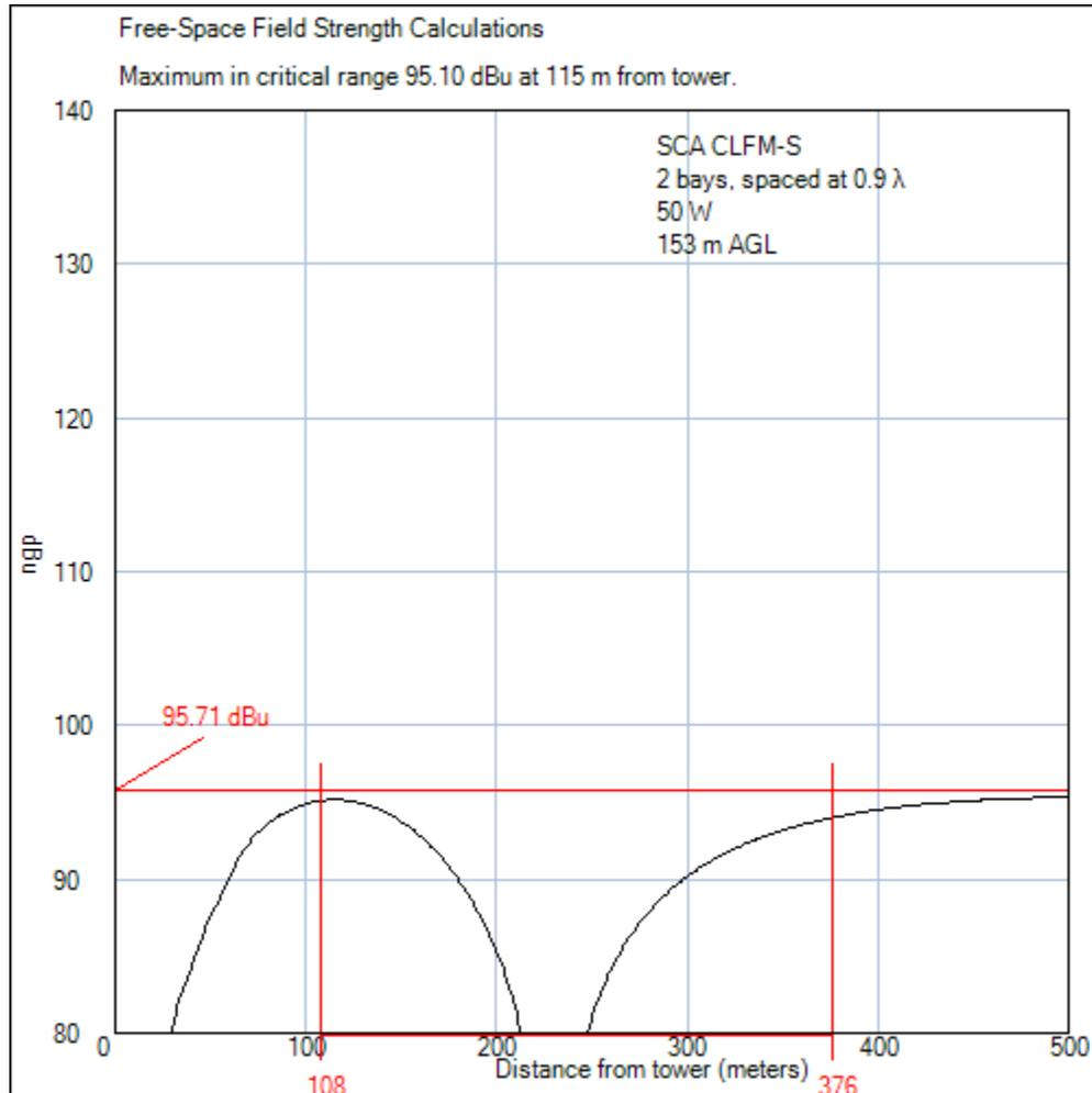
The maximum signal level anywhere in the area is 95.10 dBu, which is less than the interfering signal level of 95.71 dBu.
