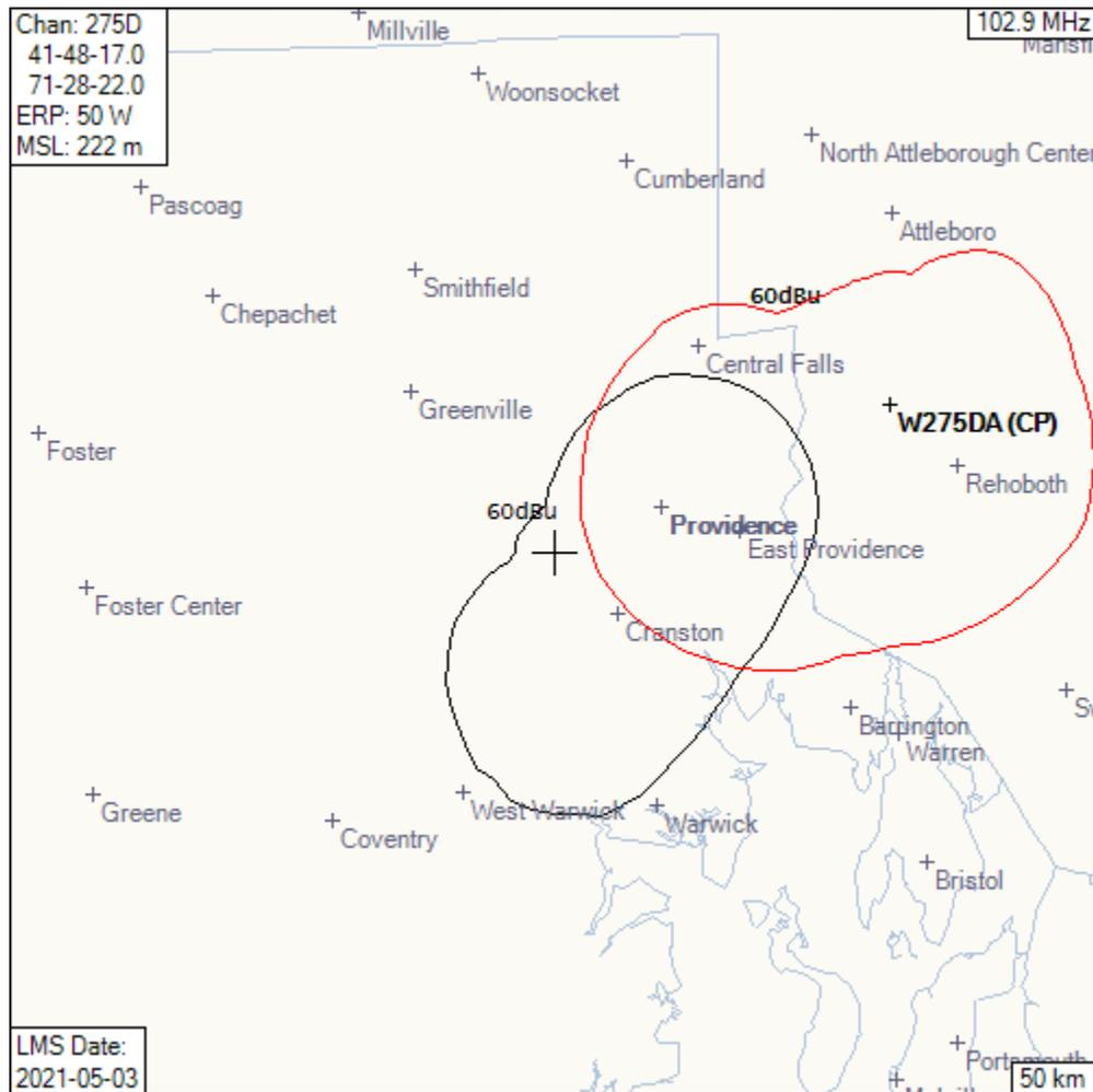
The 60 dBu f(50,50) contour of the existing Construction Permit is shown as a red polygon. The proposed 60 dBu f(50,50) contour is shown as a black polygon. The polygons intersect. No change in frequency is proposed. Therefore, the proposal qualifies as a minor change.
