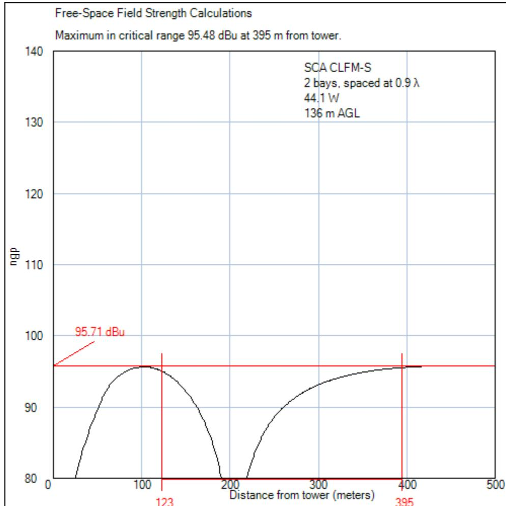
The maximum signal level in the area is 95.48 dBu, which is less than the allowable interfering signal level of 95.71 dBu.
