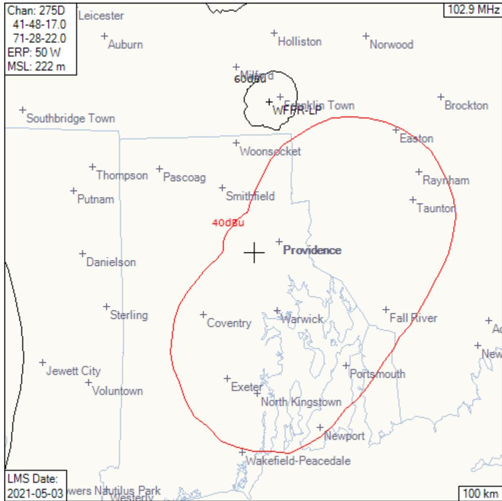
WFR-LP is Class L1, protected to the 60 dBu f(50,50) contour. The proposed interfering 40 dBu f(50,10) contour does not intersect the WFR-LP protected contour.
