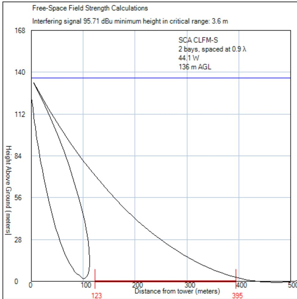
The interfering signal level of 55.71 dBu is at least 3.6 m above ground anywhere in this area.
