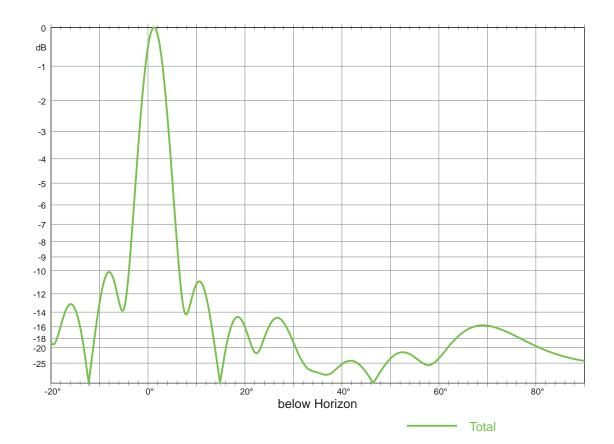
Antenna, Order No. 75010300 Number of Bays: 4 Frequency: 557 MHz Elevation Directivity: 9.22 dBd
