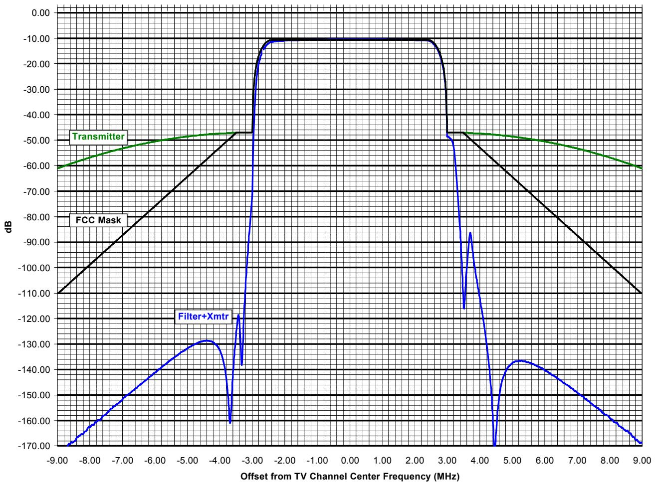
As shown above, a cascaded filter adds significant attenuation to OOB beginning at -3 MHz which is the lower end of TV channel 20. Combined with the transmitter pre-filter response, very effective filtering of OOB is provided and surpasses that of the full-service FCC mask.
