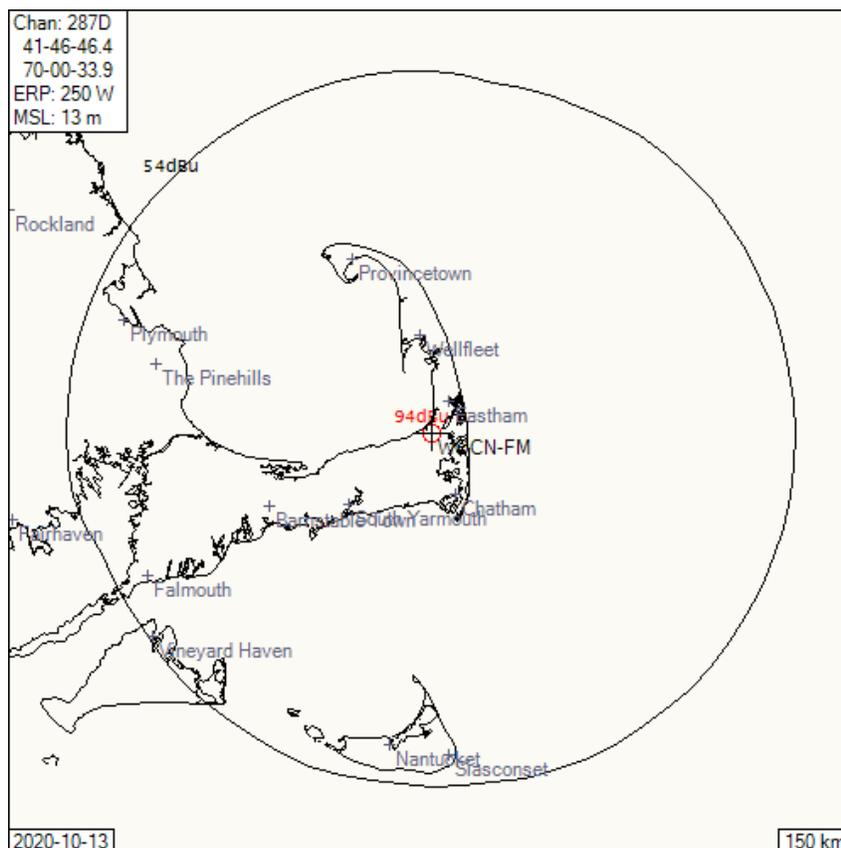
The WOCN signal at the proposed site is approximately 143 dBu. The +40 U/D interfering signal is 183 dBu. At the proposed 250 W ERP, the distance to the interfering signal level is 0.1 m, about 4". It is self-evident that interference to WOCN will not occur in any habitable area.
